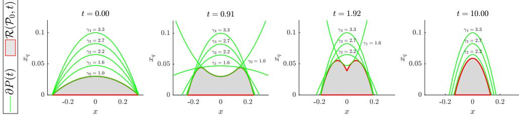
Figure 5: Time-varying paraboloids overapproximate the reachable set at different time instants  $t$  in  $\{0.00, 0.91, 1.62, 10.00\}$  for different initial conditions  $P_i(0) = \gamma_i \mathcal{P}_0$ , where scaling factors  $\gamma_i$  are respectively equal to 1.0, 1.6, 2.2, 2.7 and 3.3 for  $i = 0, \dots, 4$ . The shaded regions are the reachable set  $\mathcal{R}(\mathcal{P}_0, t)$ , the thin green lines are the boundary of the overapproximation  $P(t)$  of Theorem 1.
