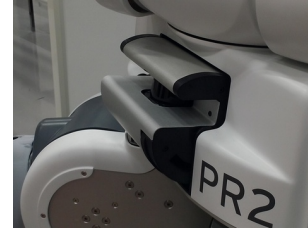
Fig. 2. The tilting LRF mounted of the PR2 robot.
