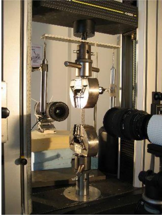
Figure 23: Pin pull-out from laminate test assembly
