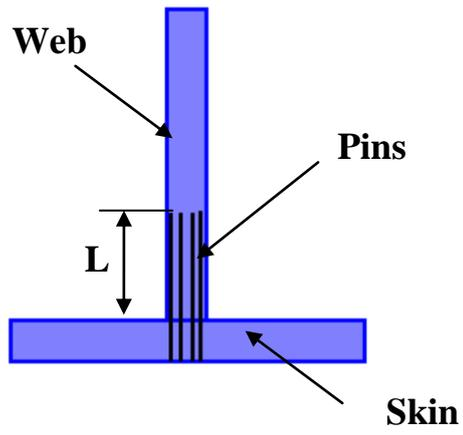
Figure 20: Typical T-Joint.
