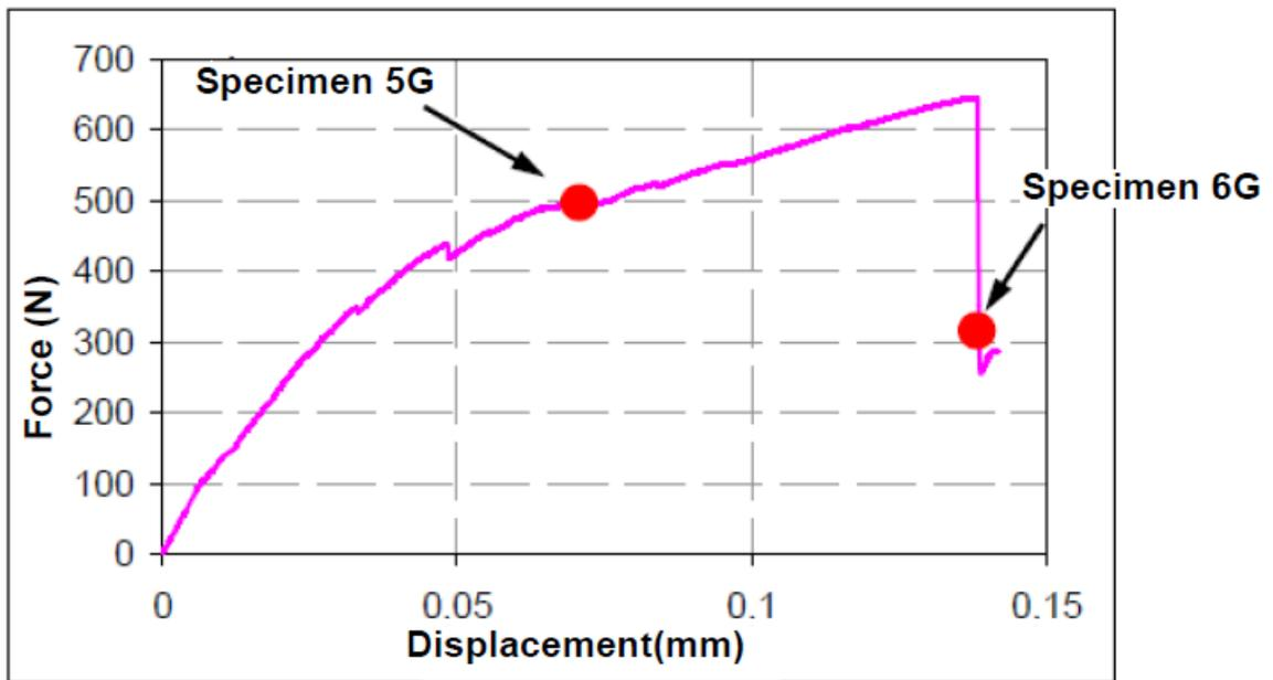
Figure 24: Typical load/displacement curve of pin pull-out from laminate
