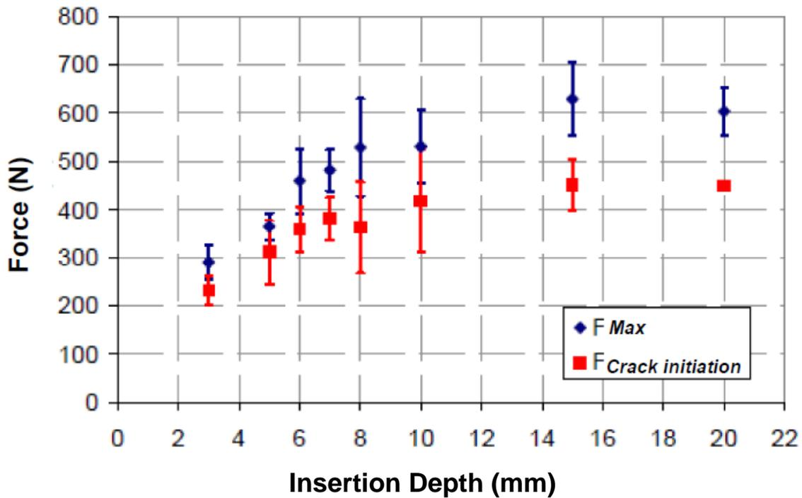
Figure 27: Crack initiation load (red) and maximum applied load (blue). Pin pull-out from laminate
