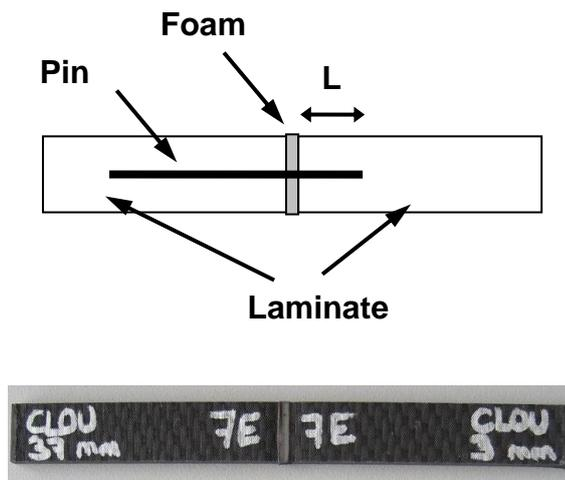
Figure 21: Pin inside laminate: Pull-out specimen diagram principle.
