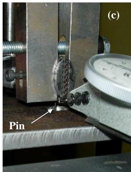
Figure 11: Pull-out test of a single pin in net resin: (a) principle, (b) test device, (c) zoom on the grips.
