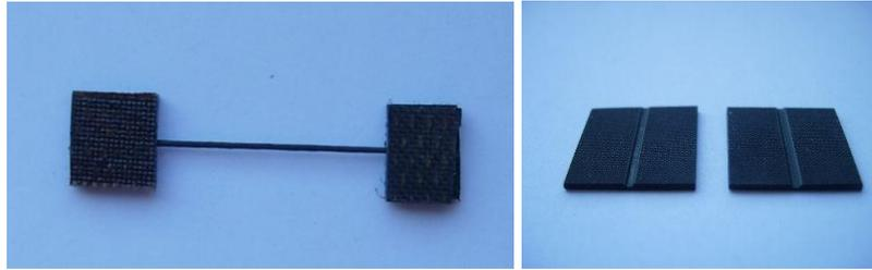
Figure 6: Single pin specimen with loading plates.
