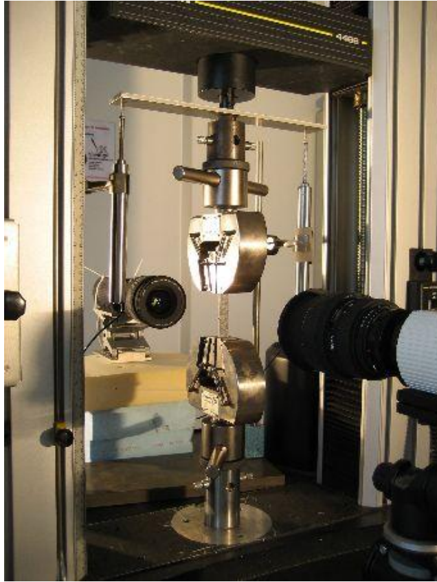
Figure 23: Pin pull-out from laminate test assembly
