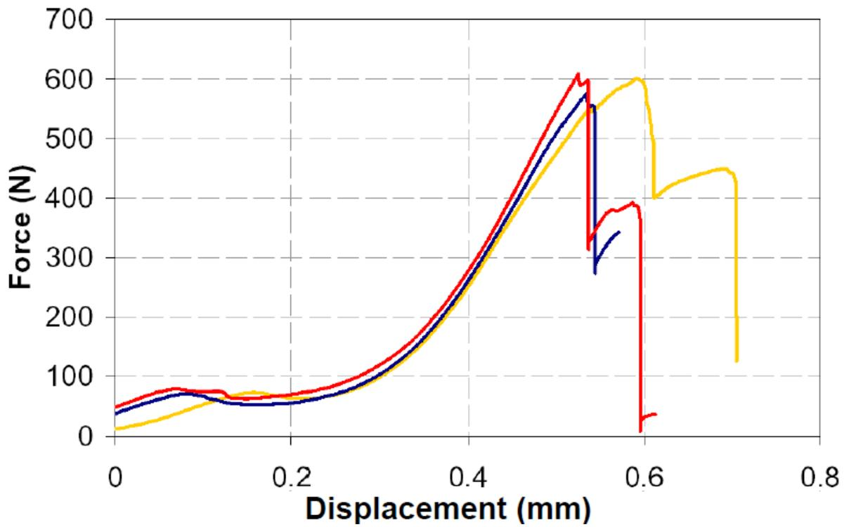
Figure 9: Shear tests force/displacement curves for 0.7 mm pins.
