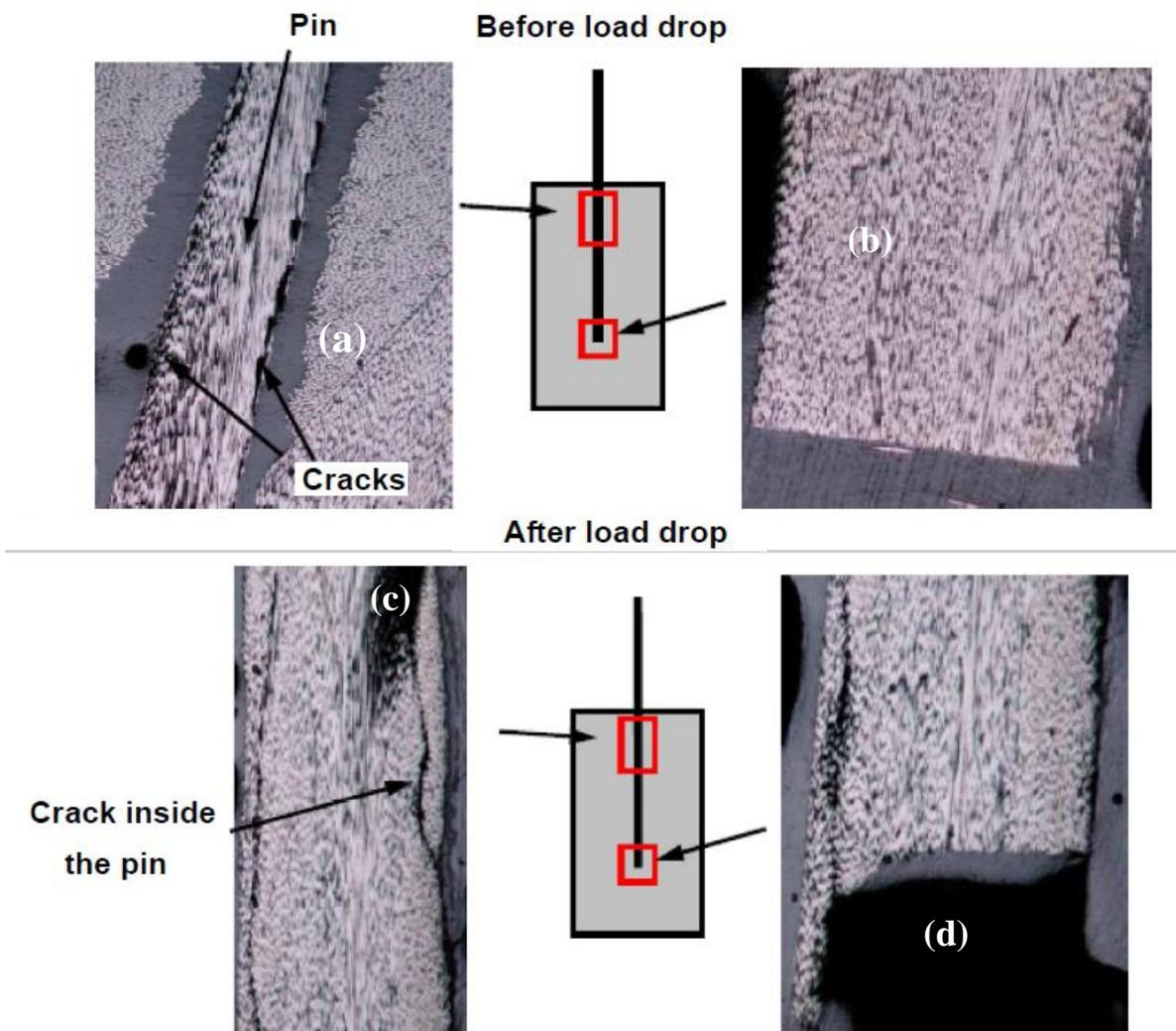
Figure 25: Micrographic analysis before (top) and after (bottom) load drop
