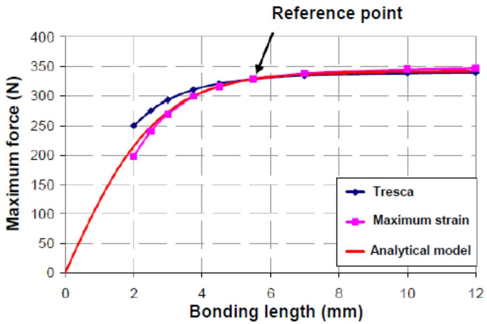
Figure 19: Comparison of shear stress and debonding load found by FEA with analytical results.
