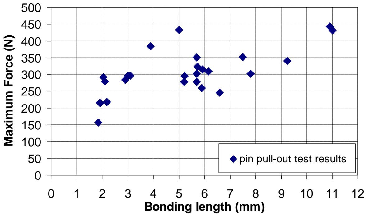
Figure 13: Experimental pin pull-out strength values.
