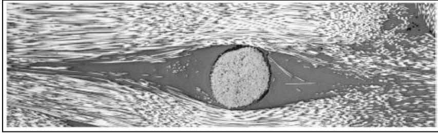
*Figure 1: Resin pocket around a pin (reproduced from [7]).*
