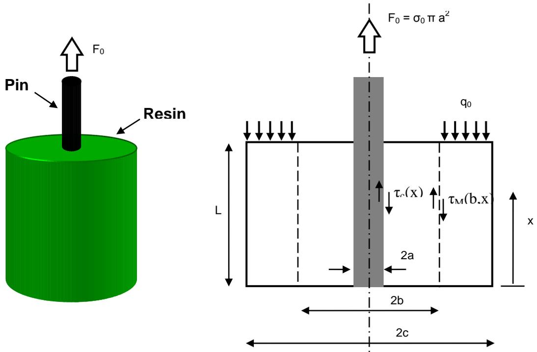
Figure 16: Modelling Z-pin pull-out.
