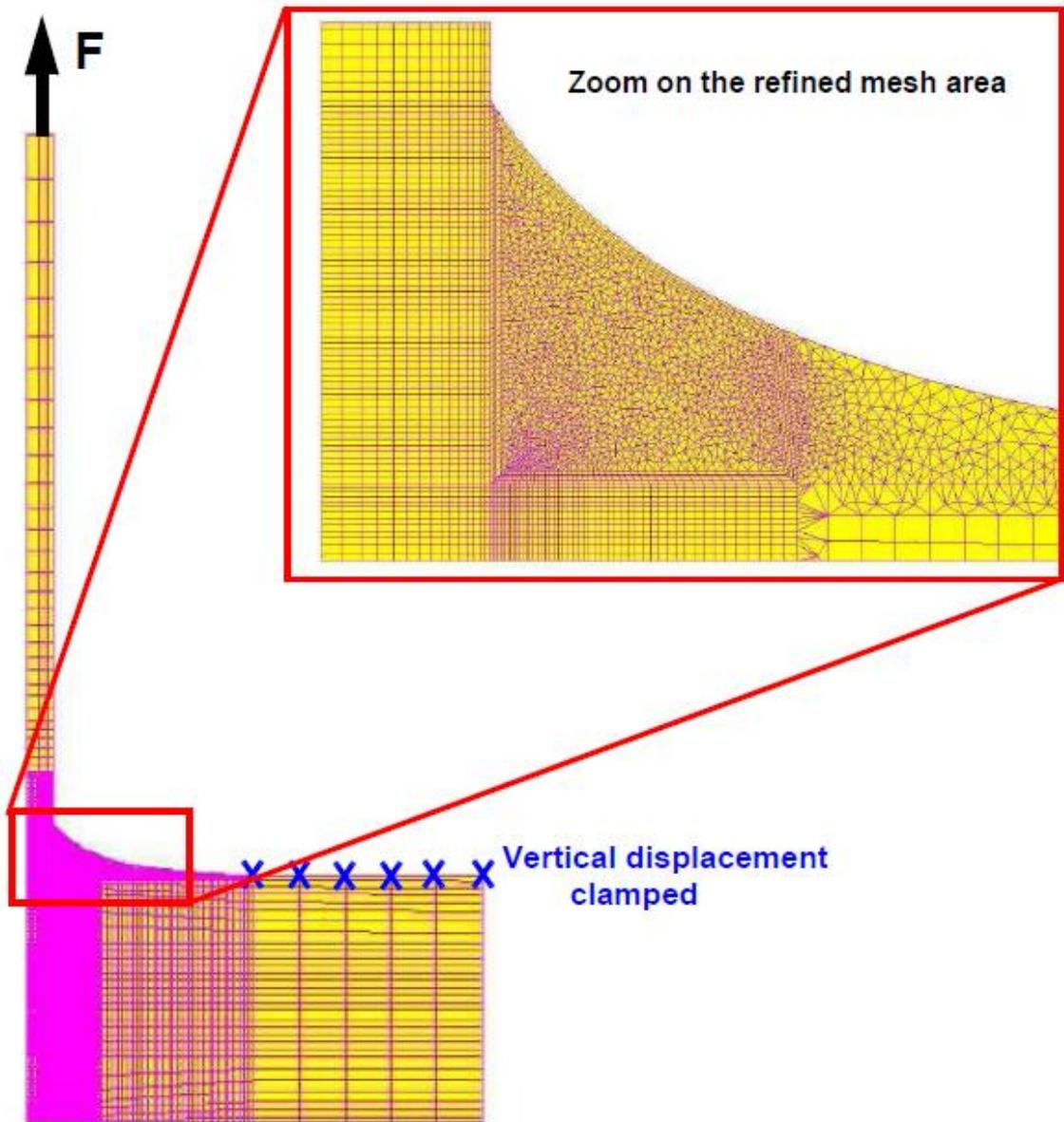
Figure 18: Detailed Finite Element model
