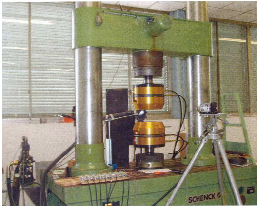
(a) 160 kN compression test machine
