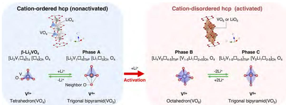
**Figure 5.** Overall redox mechanism of  $\text{Li}_3\text{VO}_4$  without (left) and with (right) activation process. Without activation, the accommodation of the reversible  $5+/4+$  vanadium valence state is ensured by a shift out of the center of the Td environment. With activation the reduction down to  $\text{V}^{3+}$  induce irreversible migration of V to Oh sites and further delithiation/lithiation proceed mainly via local distortion.
