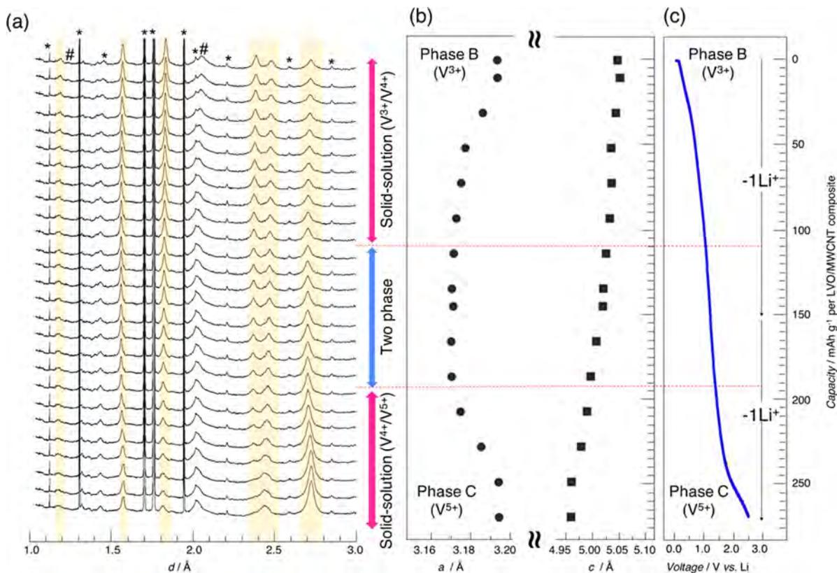
**Figure 3.** (a) Synchrotron in operando XRD patterns for uc-Li<sub>3</sub>VO<sub>4</sub>/MWCNT (60/40) collected during the delithiation at 20 cycles (\* in situ cell Bragg peaks and # MWCNT Bragg peaks) with (b) refined *a* and *c* cell parameters and (c) electrochemical curve.
