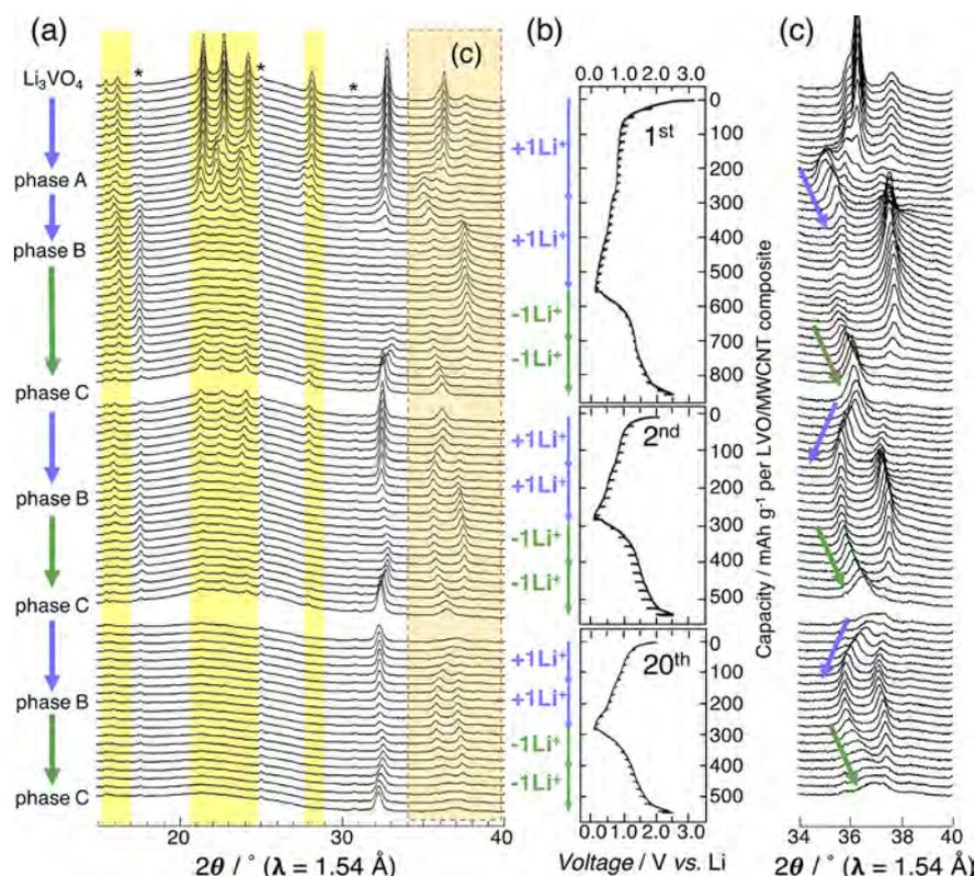
**Figure 2.** (a) In situ XRD patterns for (uc-Li<sub>3</sub>VO<sub>4</sub>/MWCNT (60/40)) at the 1st, 2nd, and 20th cycles along with (b) corresponding lithiation–delithiation curves. (c) Magnified XRD patterns within the 2θ region between 34° and 40°.
