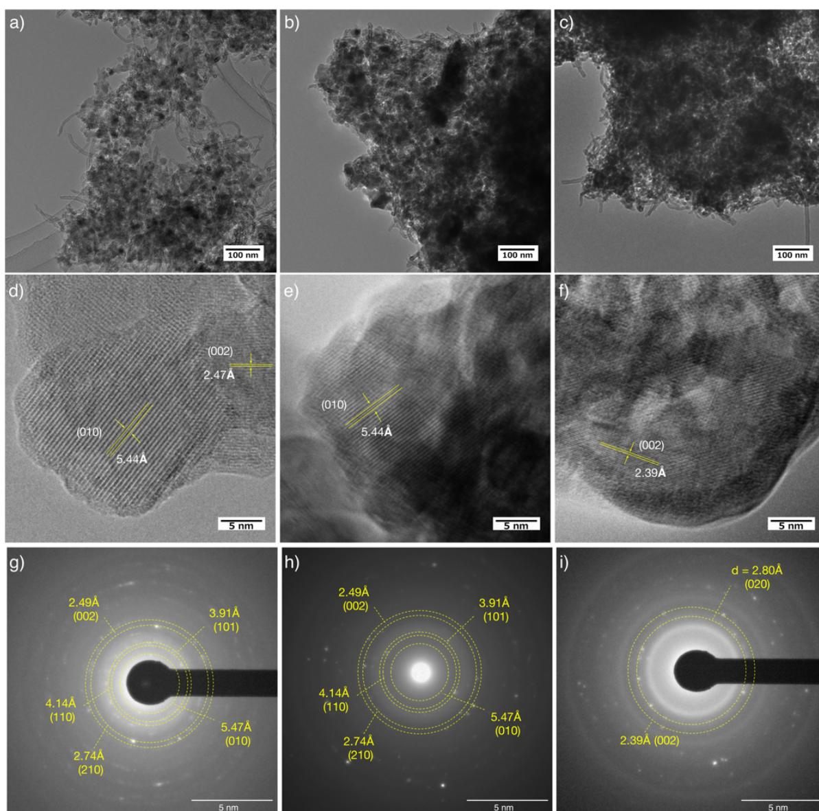
**Figure S2** TEM images focused on composite morphology (a)-(c) and crystalline lattice (d)-(f) and ED patterns (g)-(i) for different three samples; pristine  $\text{Li}_3\text{VO}_4/\text{MWCNT}$  (a), (d), (g), nonactivated  $\text{Li}_3\text{VO}_4/\text{MWCNT}$  (b), (e), (h), and activated  $\text{Li}_3\text{VO}_4/\text{MWCNT}$  (c), (f), (i); activation condition: cycling 20 times at  $0.1 \text{ A g}^{-1}$  between 0.1 and 2.5 V.
