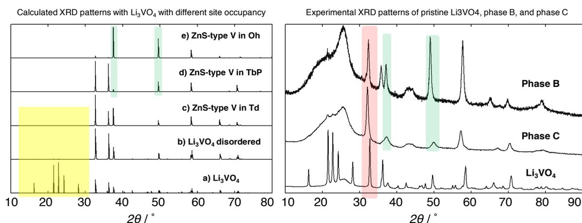
**Figure S4 [Left]** (a)-(e) calculated XRD patterns for  $\text{Li}_3\text{VO}_4$  with different site occupancy. **[Right]** Experimental XRD patterns of pristine  $\text{Li}_3\text{VO}_4$ , phase C, and phase B. The diffraction angles were recalculated in  $\lambda\text{CuK}\alpha$  for the easy comparison.
