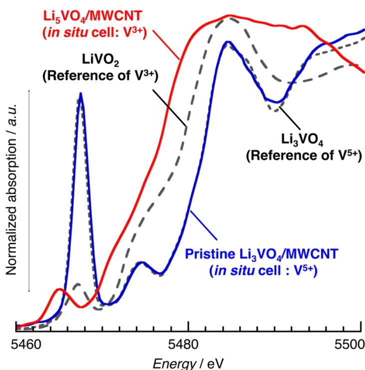
**Figure S5.** XANES spectra for the pristine Li<sub>3</sub>VO<sub>4</sub>/MWCNT (V<sup>5+</sup>) and Li<sub>5</sub>VO<sub>4</sub>/MWCNT (V<sup>3+</sup>) in the *in situ* laminate type cell at 1<sup>st</sup> cycle, along with the spectra for reference powder samples; Li<sub>3</sub>VO<sub>4</sub>(V<sup>5+</sup>) and LiVO<sub>2</sub>(V<sup>3+</sup>).
