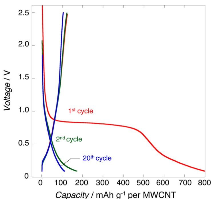
**Figure S1.** Charge / discharge curves at 0.04 A g<sup>-1</sup> for uc-MWCNT during 1<sup>st</sup> (red), 2<sup>nd</sup> (green), and 20<sup>th</sup> (blue) cycles. The cell contains 10 mg of MWCNT powder (cathode) and a Li metal (anode). One layer of 420  $\mu$ m-thick glass fiber separator (Nippon Kodoshi) was used as a separator. The voltage was set from 0.1 V to 2.5 V vs Li after the initial lithiation.
