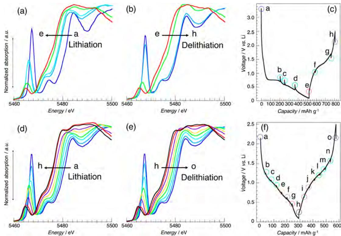
**Figure 4.** In situ XANES spectra recorded during lithiation (a) and delithiation (b) of a uc-Li<sub>3</sub>VO<sub>4</sub>/MWCNT sample at the 1st cycle and corresponding charge–discharge curves (c). XANES spectra of lithiation (d) and delithiation (e) for the same uc-Li<sub>3</sub>VO<sub>4</sub>/MWCNT sample at the 20th cycle and its corresponding charge–discharge curve (f).
