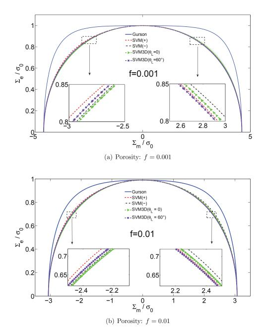
Figure 2: Comparison between the yield surfaces obtained from the established criterion SVM3D (35) with axisymmetric trial stress field, the closed form criterion of Stress Variational Model (SVM(+) and SVM(-)) (Cheng et al., 2013) and the Gurson criterion (Gurson, 1977). Porosity: f = 0.001 and f = 0.01.
