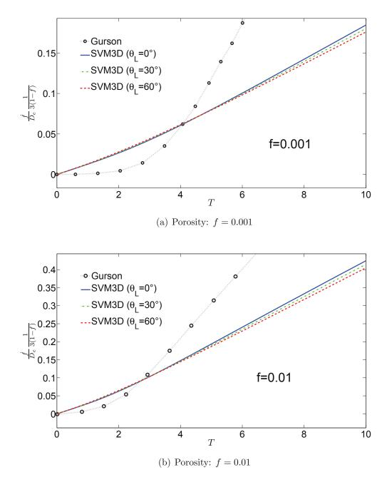
Figure 3: Evolution of porosity as function of the stress triaxiality for initial porosity f = 0.001 and f = 0.01 with three values of Lode angle:  $\theta_L = 0$ , 30° and 60°.
