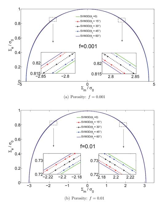
Figure 1: Illustrations of the yield surfaces obtained from the new established criterion SVM3D (35) with five values of Lode angle:  $\theta_L = 0, 15^{\circ}, 30^{\circ}, 45^{\circ}$  and  $60^{\circ}$ . Porosity: f = 0.001 and f = 0.01.
