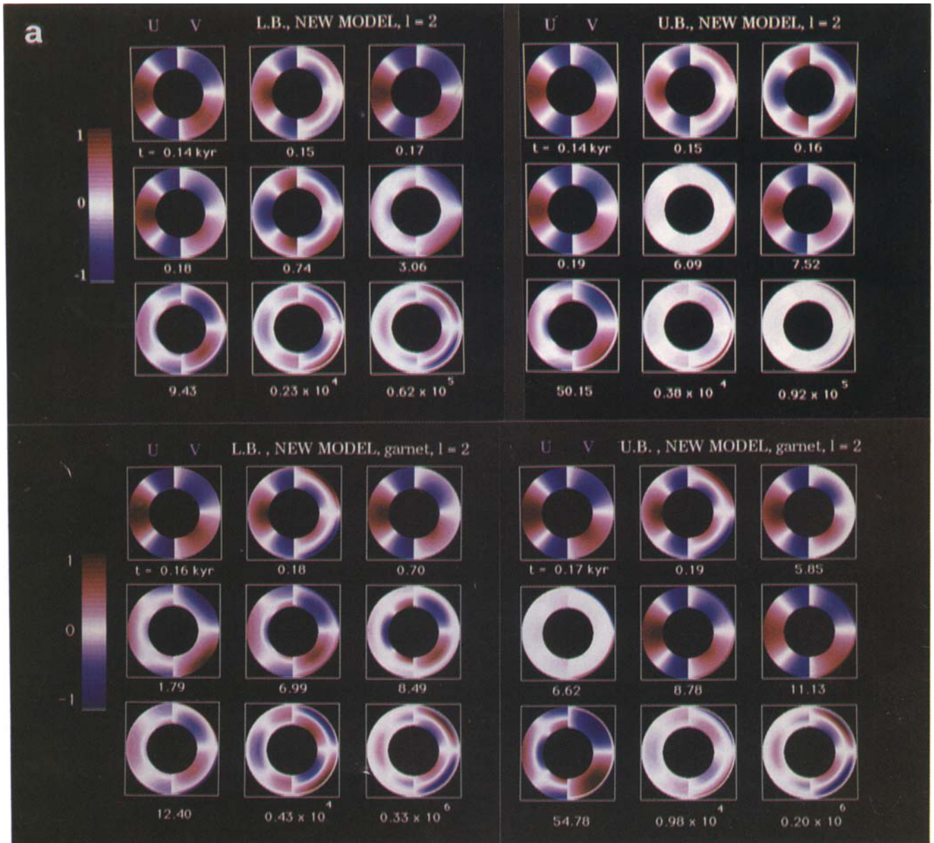
Figure 4. New model NM. For the l=2 and l=9 harmonic loading, (a) and (b) respectively, the radial and tangential components of the displacement for each of the nine modes carried by the five-layer model are portrayed. The modes are ordered as a function of their relaxation time in kyr. The left portion of the ring corresponds to the radial component U while the right portion corresponds to the tangential component V. The amplitude of each mode is normalized to one. The colour palette has 25 evenly spaced intervals and is linear in magnitude. The lower and upper mantle viscosities are varied as shown in Table 2 for the lower and upper branches LB, UB respectively. In the first two panels on the top only the lower mantle viscosity is varied, while in the last two panels at the bottom, the effects of a viscosity increase in the hard layer with C = 50 are considered.
