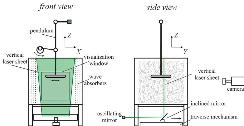
FIGURE 1. Sketch of the experimental set-up: (a) front view and (b) side view with the seeded particles as light grey dots and the laser plane shown in green.
