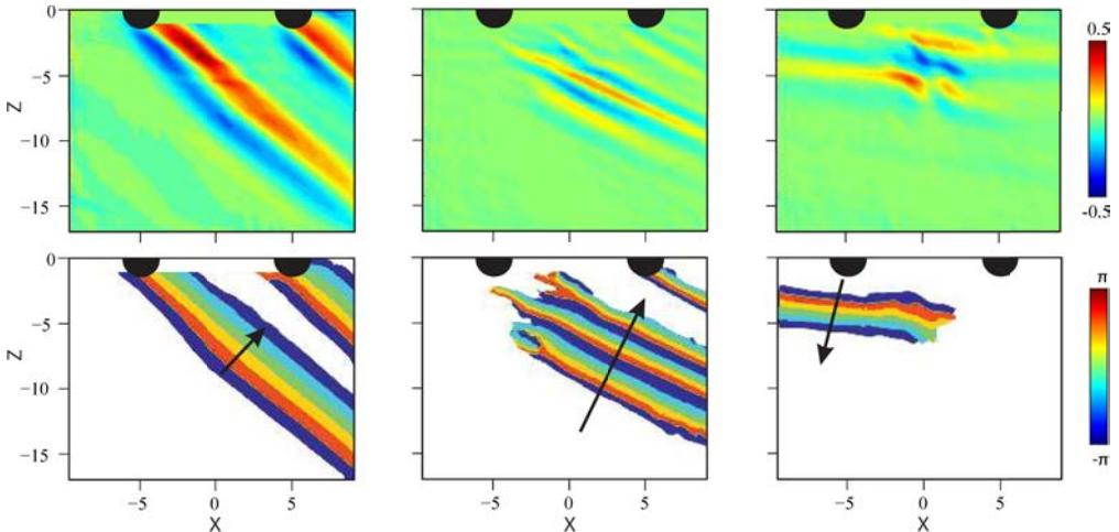
FIGURE 6. Hilbert decomposition in time and space of instantaneous horizontal velocity profile (upper row) and phase velocity (lower row) for  $Fo = 0.33$ . (a,d) First harmonic  $U^1$  with frequency  $\omega^1/N = 0.8$  and  $k > 0$ ; subharmonics with (b,e)  $\omega_1/N = 0.6$ ,  $k > 0$ , and (c,f)  $\omega_2/N = 0.2$ ,  $k < 0$ . (Exp. E from table 1)
