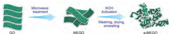
Figure 3. A scheme shows the microwave exfoliation/reduction of GO and the following chemical activation of GO with KOH. MEGO = microwave-exfoliated graphene oxide.
