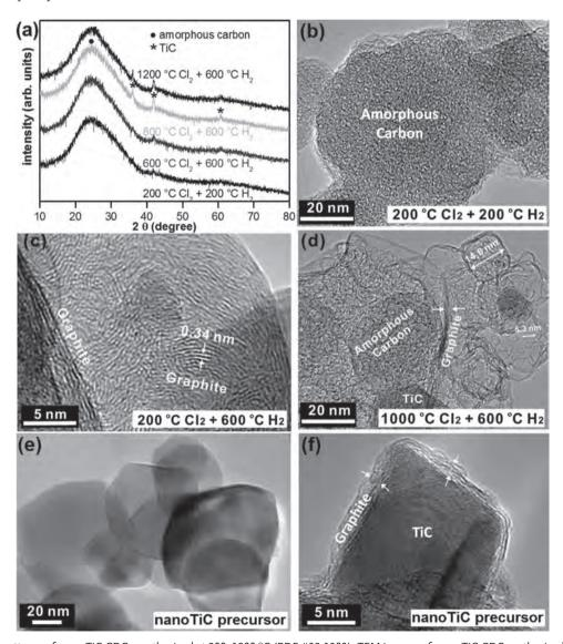
Figure 1. a) XRD patterns of nano-TiC-CDCs synthesized at 200–1200  $^{\circ}$ C (PDF #32-1383). TEM images of nano-TiC-CDC synthesized and H<sub>2</sub>-annealed at indicated temperatures (b–d) and nano-TiC precursor (e,f).
