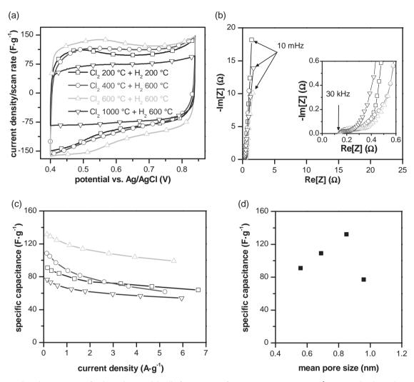
Figure 5. a) Cyclic voltammograms of 3-electrode Swagelok cell of nano-CDCs of various pore sizes at 5 mV  $s^{-1}$  scan rate. b) Electrochemical impedance spectroscopy (EIS) of nano-CDCs of various pore sizes. c) Specific capacitance as a function of current density during galvanostatic cycling of nano-CDCs of various pore sizes in a three-electrode cell. d) Specific capacitance versus pore size of nano-CDC samples.
