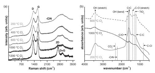
Figure 2. a) Raman and b) FTIR spectra of nano-CDCs synthesized at 200–1200 °C with subsequent hydrogen annealing. Nano-CDCs synthesized at 200 and 400 °C were annealed the same temperatures. All other samples were annealed at 600 °C. The Raman spectra were normalized to the intensity of the G-band at 1582 cm<sup>-1</sup> and shifted along the Y-axis for clarity.
