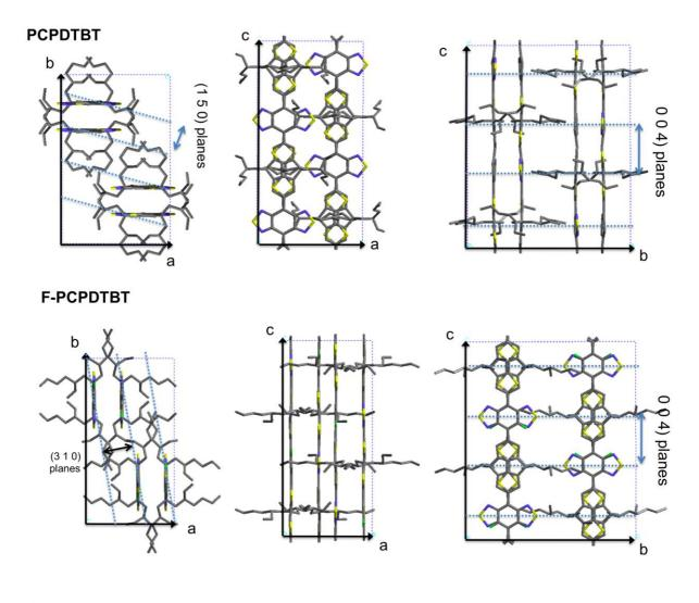
**Figure 4**. Projections along the a,b and c unit cell axes of the structural models refined from the ED data shown in figure 1 and 2 for PCPDTBT and F-PCPDTBT.
