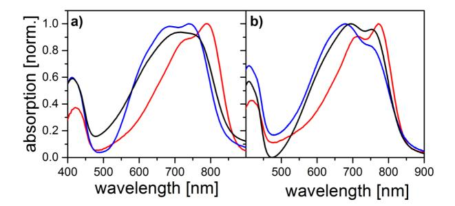
**Figure 3** Absorption spectra of thin films prepared by different techniques. **a**) PCPDTBT absorption spectra of thin films prepared by spin coating from CB/DIO (2w%, red), CB-annealing (blue) and melt-annealing on PTFE (black). **b**) F-PCPDTBT absorption spectra of thin films prepared by spin coating from CB/DIO (2w%, red), CB-annealing (blue) and high temperature rubbing (240°C, black).
