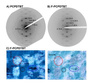
**Figure 5**. a) and b) show ED patterns taken from the highly crystalline almost transparent areas shown in the transmission polarized microscopy images of F-PCPDTBT in Figure c and
