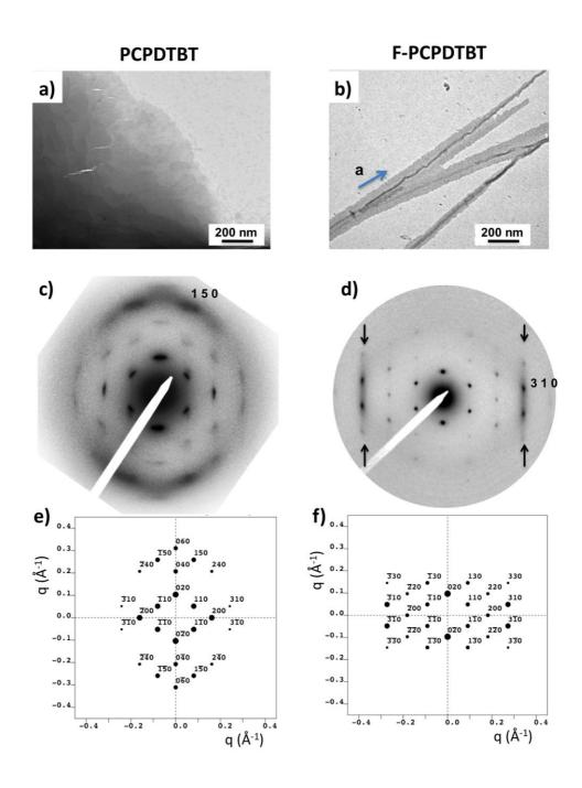
**Figure 1**. Bright field images (a, b), experimental ED patterns (c, d) and calculated ED patterns for the [0 0 1] zone (e, f) for PCPDTBT and F-PCPDTBT using the refined structural models shown in figure 4. The arrows in Figure 1.d highlight the streaked reflections in the ED pattern of the F-PCPDTBT crystals.
