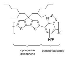
Scheme 1. Chemical structures of PCPDTBT and F-PCPDTBT.
