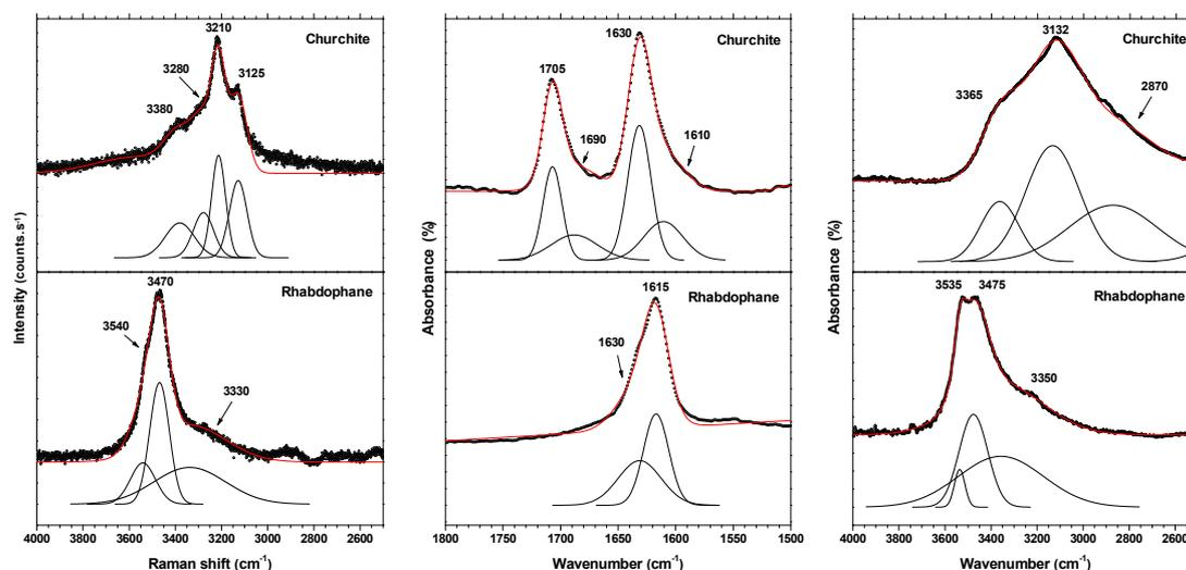
**Figure 8.** Raman spectra in the  $2500\text{-}4000\text{ cm}^{-1}$  range and FTIR spectra in the  $1500\text{-}1800\text{ cm}^{-1}$  and  $2500\text{-}4000\text{ cm}^{-1}$  regions, recorded for gadolinium rhabdophane, monazite, churchite and monazite.
