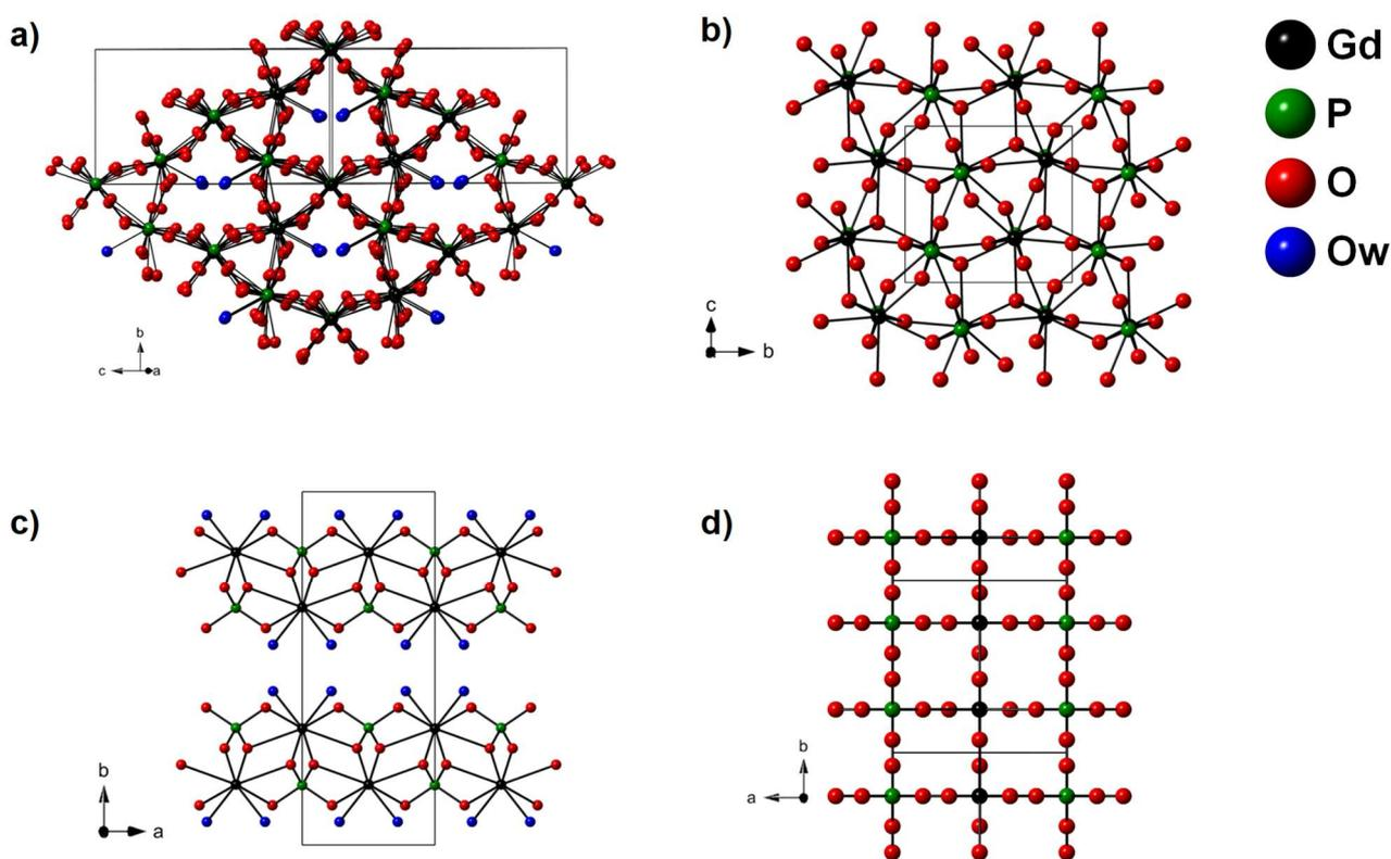
**Figure 2.** View of the structure of : a) GdPO<sub>4</sub>·0.667 rhabdophane (along the [101] direction); b) GdPO<sub>4</sub> monazite ([100] direction); c) GdPO<sub>4</sub>·2H<sub>2</sub>O churchite ([001] direction); d) GdPO<sub>4</sub> xenotime ([001] direction).
