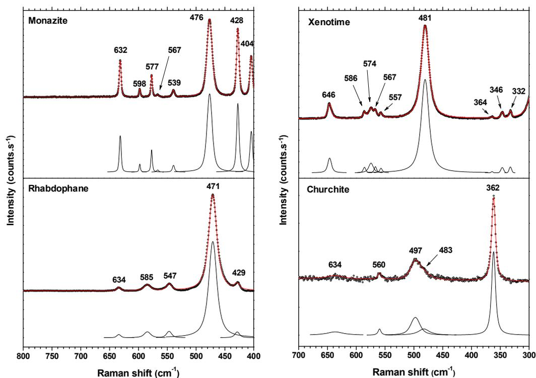
**Figure 6.** Raman spectra recorded in the 400-800  $\text{cm}^{-1}$  range for gadolinium based rhabdophane and monazite and between 300 and 700  $\text{cm}^{-1}$  for gadolinium based churchite and monazite.
