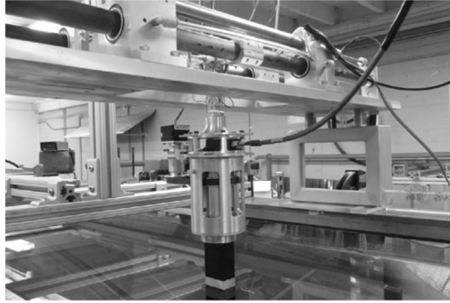
Fig. 5. Rotor rig view from the water surface level.
