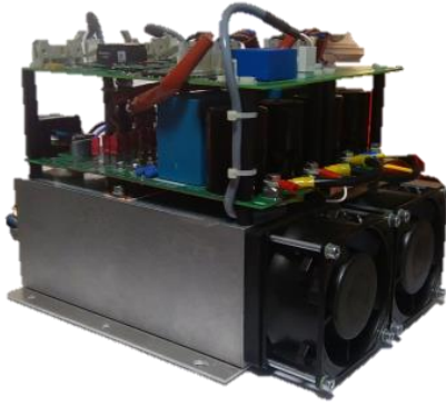
Fig. 1: Power converter prototype (ARCEL)
