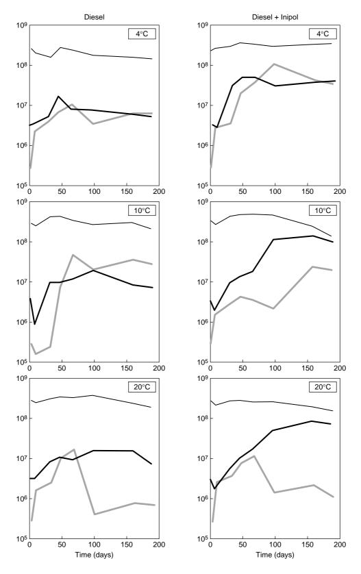
Figure 2 Changes of microflora composition during incubation of the diesel oil-contaminated mesocosms (thin line: total cells in cell  $mL^{-1}$ ; bold line: viable cells in CFU  $ml^{-1}$ ; gray line: hydrocarbon-degrading cells in MPN  $ml^{-1}$ ).
