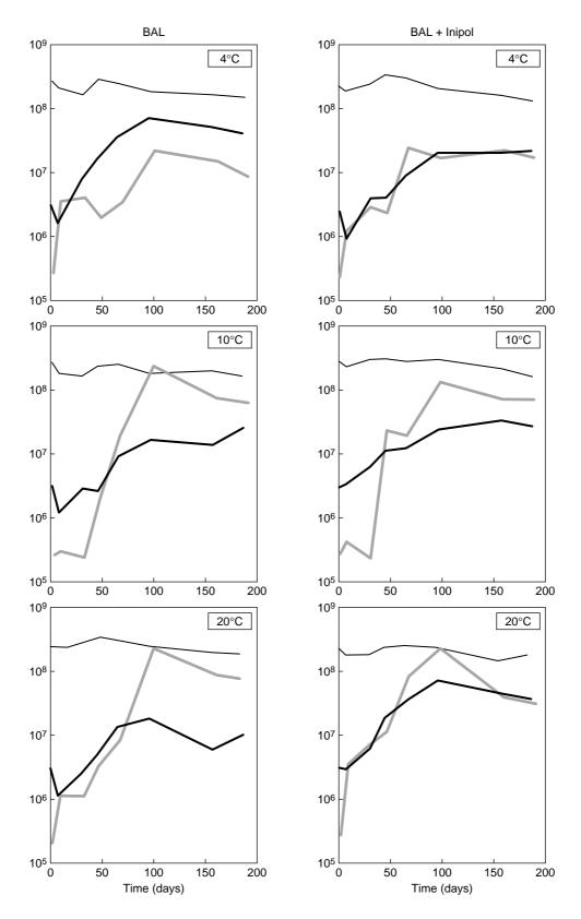
Figure 3 Changes of microflora composition during incubation of the crude oil contaminated mesocosms (thin line: total cells in cell ml<sup>-1</sup>; bold line: viable cells in CFU ml<sup>-1</sup>; gray line: hydrocarbon-degrading cells in MPN ml<sup>-1</sup>).
