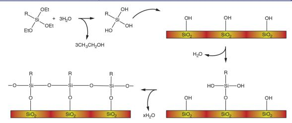
Figure 1. Illustration of lateral self-condensation of triethoxysilanes on a silica surface, eventually forming a perfectly condensed monolayer.
