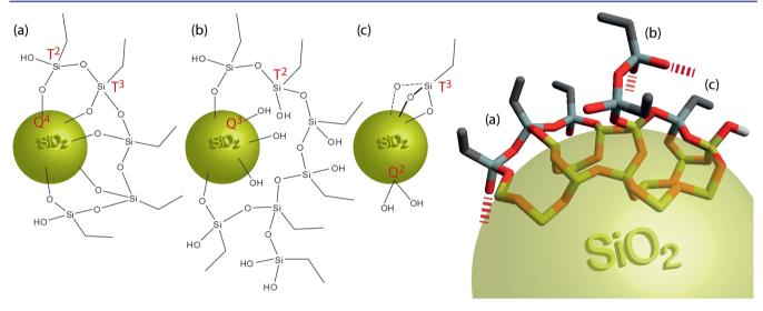
Figure 2. 2D (left) and 3D (right) schematics representing surface grafting possibilities for organosiloxanes on silica: (a) laterally self-condensed on the surface, (b) vertical core—shell oligomers above the surface, (c) discrete surface-bound monomers. The nanoparticle Si, silane Si, O, C, and H atomic environments are presented as yellow, light gray, red, dark gray, and white colors, respectively.
