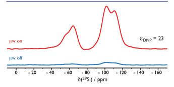
**Figure 3.** Illustration of the signal enhancement from DNP via 1D  ${}^{1}\text{H-}{}^{29}\text{Si}$  CPMAS spectra of the PES-functionalized silica NPs, recorded using conditions suitable for DNP with (red) and without (blue) microwave irradiation.
