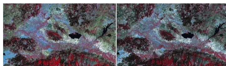
Fig: Fragments of classified Landsat TM 2000 image (full AOI area), illustrating two classification methods: 'Maximal Likelihood' (left) and 'Minimal Distance' (right)
