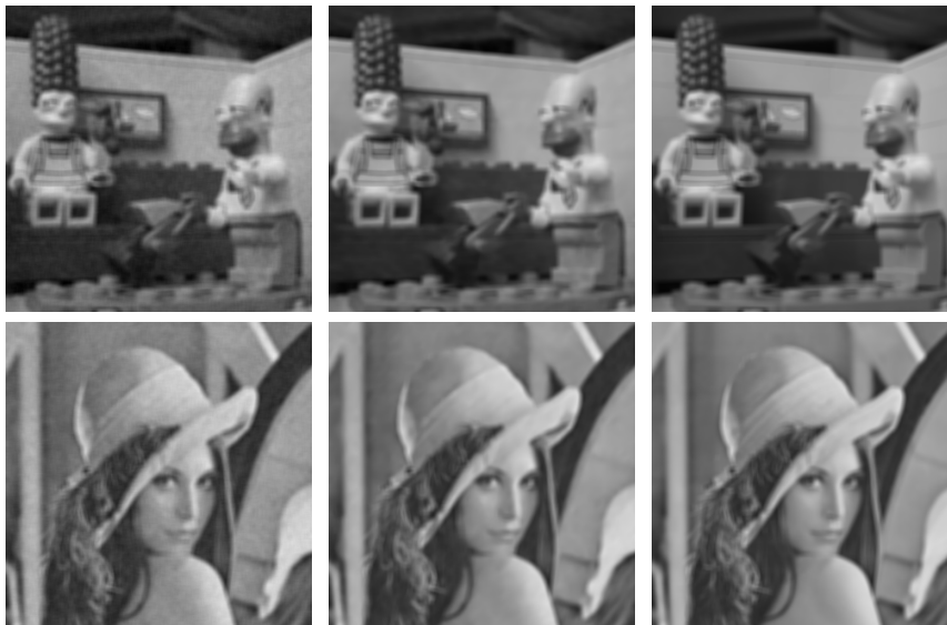
Figure 2: Left: noisy DC image. Middle: denoised DC image ('simpson' PSNR = 40.64 dB , 'lena' PSNR = 40.89 dB). Right: oracle DC image. Top line is the from the simpson image and bottom line from the lena image both with noise of standard deviation \sigma = 30/255 .
