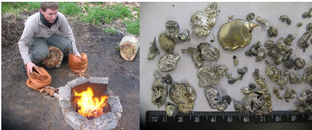
Fig. 12: (left) Experimental tin smelting operation performed in an open pit recreating prehistoric technologies; (right) tin prills recovered from the smelting experiment.
