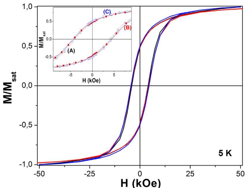
**Figure 7.** Variation of the normalized zero field cooling magnetization as a function of the magnetic field measured at 5 K on (A) Co<sub>0.6</sub>Zn<sub>0.4</sub>Fe<sub>2</sub>O<sub>4</sub>, (B) Co<sub>0.6</sub>Zn<sub>0.4</sub>Fe<sub>1.98</sub>Gd<sub>0.02</sub>O<sub>4</sub>, and (C) Co<sub>0.6</sub>Zn<sub>0.4</sub>Fe<sub>1.94</sub>Gd<sub>0.06</sub>O<sub>4</sub> nanoparticles dispersed in an alumina matrix.
