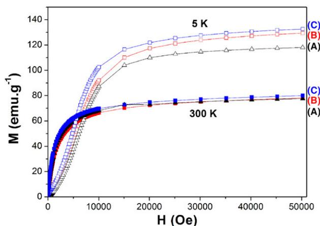
**Figure 8.** First magnetization curves recorded at 300 and 5 K on (A) Co<sub>0.6</sub>Zn<sub>0.4</sub>Fe<sub>2</sub>O<sub>4</sub>, (B) Co<sub>0.6</sub>Zn<sub>0.4</sub>Fe<sub>1.98</sub>Gd<sub>0.02</sub>O<sub>4</sub>, and (C) Co<sub>0.6</sub>Zn<sub>0.4</sub>Fe<sub>1.94</sub>Gd<sub>0.06</sub>O<sub>4</sub> nanoparticles dispersed in an alumina matrix.
