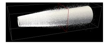
**Figure 2.** Measurement plane located at 5 diameters from the nozzle, represented by 4 red edges along with droplets colored as white dots.
