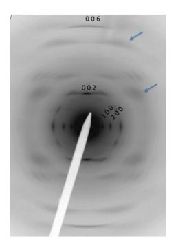
**Figure S5**. Electron diffraction pattern of a highly crystalline and oriented P3HT film obtained by high-temperature rubbing at  $180^{\circ}$ C. The two arrows point at fuzzy reflections indicative of structural disorder in the packing of n-hexyl side chains in form I P3HT.
