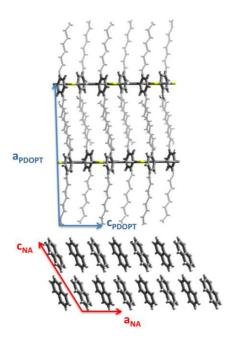
**Figure 7**. Structural model showing the section profile of the  $(1\ 0\ 0)_{PDOPT}/(0\ 0\ 1)_{NA}$  interface. Note the epitaxial growth condition  $\mathbf{c}_{PDOPT}//a_{NA}$  with  $|\mathbf{c}_{PDOPT} - \mathbf{a}_{NA}|/\mathbf{c}_{PDOPT} \approx 4\%$  indicating that orientation of PDOPT chains is due to the 1D epitaxial orientation of the n-octyl side chains on NA.
