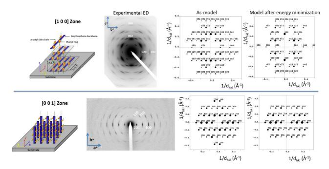
**Figure 8**. Comparison of the experimental electron diffraction patterns of highly oriented PDOPT films (6 kDa) grown by slow-DEC on naphthalene corresponding to the [1 0 0] and the [0 0 1] zones with the calculated ED patterns obtained for the structural model obtained by trial-and-error (as-model) and after energy minimization.
