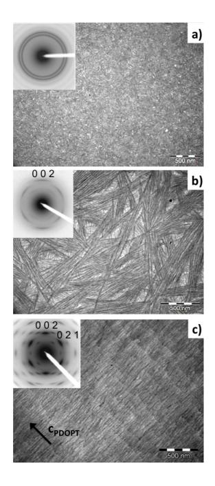
**Figure 3.** Comparison of the bright field TEM images and corresponding diffraction patterns of the PDOPT films ( $M_n$ = 21 kDa) obtained by doctor-blading from ODCB (a), isothermal crystallization at 100°C for 24 hrs (b) and epitaxy on NA (c). The arrow in (c) indicates the in-plane direction of the PDOPT chains.
