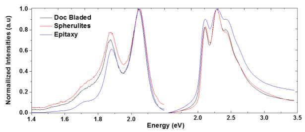
**Figure S3**. Comparison of the photoluminescence and UV-vis spectra in PDOPT films prepared by doctor blading, isothermal crystallization at 100°C and by slow directional epitaxial crystallization on naphthalene. The PL spectra are normalized with respect to the 0-0 vibronic component whereas the absorption spectra are normalized with respect to the 0-1 component.
