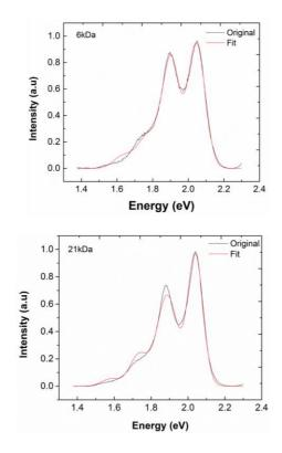
**Figure S2**. Photoluminescence spectra of oriented PDOPT films prepared by slow-DEC on naphthalene fro two different molecular weights  $(M_n)$ . The figures show the fit of the PL spectra using a simple Frank-Condon progression (in red).
