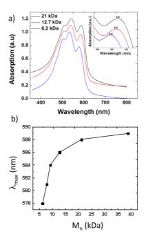
**Figure S4**. Evolution of optical absorption spectrum of PDOPT films oriented by epitaxy on naphthalene as a function of  $M_n$  (incident polarization parallel to the chain direction of PDOPT). The inset shows the shift of the 0-0 transition in the UV-vis absorption spectrum with  $M_n$ . b) Evolution of  $\lambda_{max}$  as a function of  $M_n$ .
