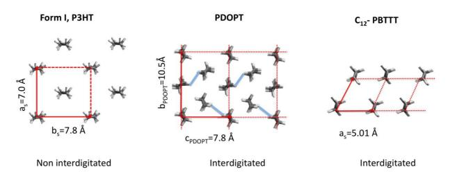
**Figure 10**. Comparison of the packing of n-alkyl side chains in polythiophene semiconductors: form I P3HT,  $^{15}$  PDOPT and C12-PBTTT. The structure of C12-PBTTT is described in reference 13. The views show the subcells formed by alkyl side chains when viewed along their long axis. For PDOPT, the phenyls linking n-octyl side chains are sketched as light blue segments.
