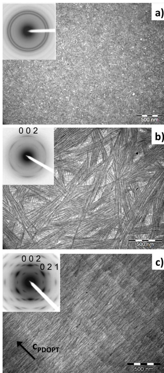
**Figure 3.** Comparison of the bright field TEM images and corresponding diffraction patterns of the PDOPT films ( $M_n = 21$  kDa) obtained by doctor-blading from ODCB (a), isothermal crystallization at  $100^\circ\text{C}$  for 24 hrs (b) and epitaxy on NA (c). The arrow in (c) indicates the in-plane direction of the PDOPT chains.
