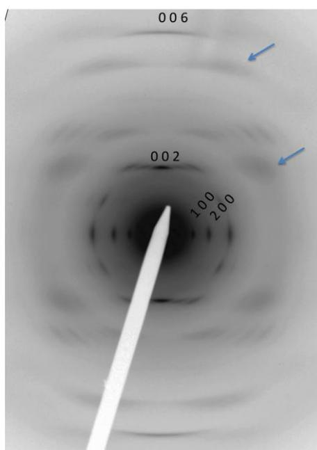
**Figure S5.** Electron diffraction pattern of a highly crystalline and oriented P3HT film obtained by high-temperature rubbing at 180°C. The two arrows point at fuzzy reflections indicative of structural disorder in the packing of *n*-hexyl side chains in form I P3HT.
