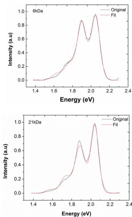
**Figure S2.** Photoluminescence spectra of oriented PDOPT films prepared by slow-DEC on naphthalene from two different molecular weights ( $M_n$ ). The figures show the fit of the PL spectra using a simple Frank-Condon progression (in red).
