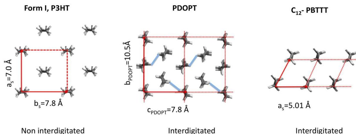
**Figure 10.** Comparison of the packing of *n*-alkyl side chains in polythiophene semiconductors : form I P3HT,<sup>15</sup> PDOPT and C12-PBTTT. The structure of C12-PBTTT is described in reference 13. The views show the subcells formed by alkyl side chains when viewed along their long axis. For PDOPT, the phenyls linking *n*-octyl side chains are sketched as light blue segments.
