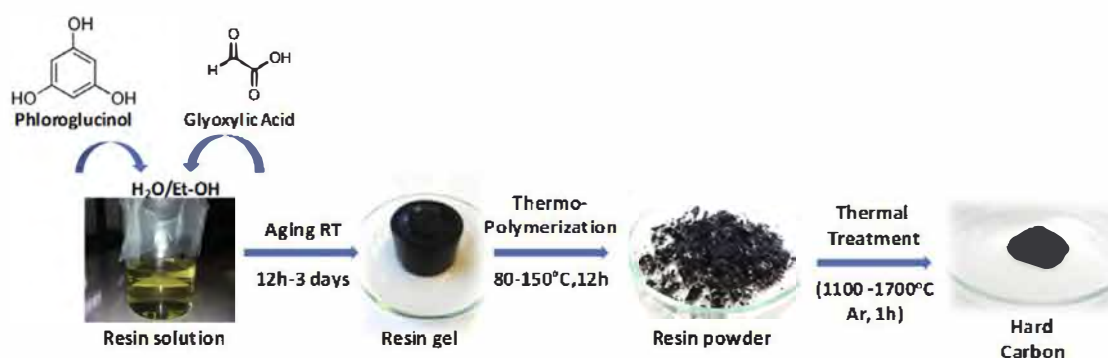
Fig. 1. Environmentally friendly synthesis procedure developed to prepare the hard carbon materials using phloroglucinol/glyoxylic acid resin. (A colour version of this figure can be viewed online.)
