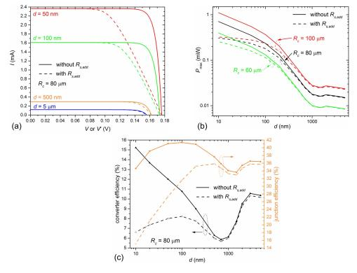
Fig. 4. Impact of the additional series resistance  $(R_{s,add})$  on: (a) current-voltage characteristics when the radius of the active part of the cell is  $R_c = 80 \ \mu\text{m}$ , (b) electrical power at the maximum power point for three values of  $R_c$ , and (c) junction and converter efficiencies when  $R_c = 80 \ \mu\text{m}$ , as a function of the vacuum gap thickness.
