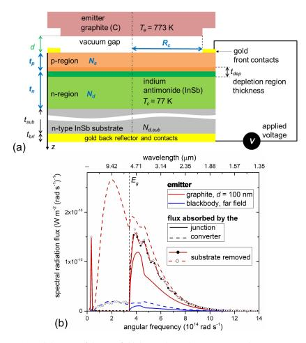
Fig. 1. (a) Schematic of the near-field thermophotovoltaic converter. The parameters to be determined for maximizing electrical power output are in blue bold font. (b) Spectral radiation flux absorbed by the p-n junction and the receiver, when the emitter is either made of graphite and the vacuum gap thickness is d = 100 nm, or a blackbody in the far field. The parameters of the p-n junction are those of case 2-1-1 described in section 3.2.
