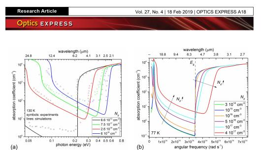
Fig. 2. Absorption coefficient of n-doped InSb as a function of doping concentration  $N_d$ : (a) at 130 K, comparison of simulations with experimental data in [54]. (b) at 77 K, impact on interband and free carrier absorption.
