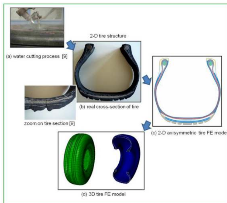
Figure 12. Tire 3-D finite element model built-up from the 2-D tire cross section.
