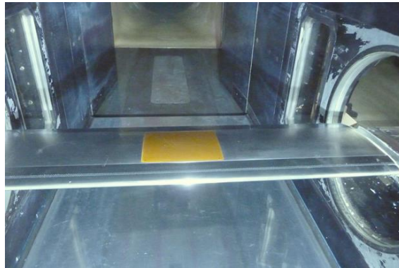
Figure 1. Picture of the model installed in the test section as viewed from upstream (leading edge facing). The yellow part is the PSP insert.
