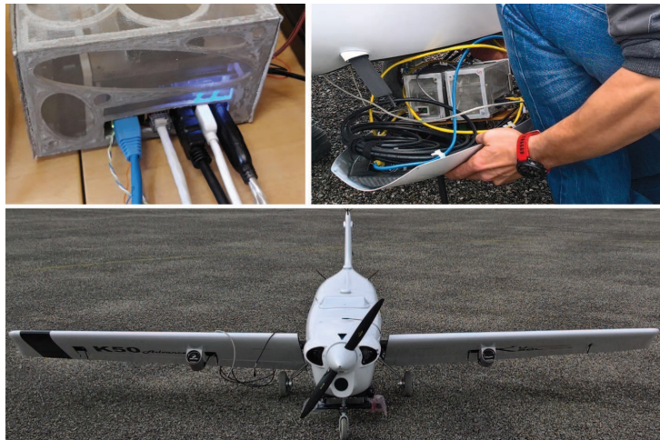
Fig. 15 Payload computers and the monocular cameras (under wings) on the K50 UAV.
