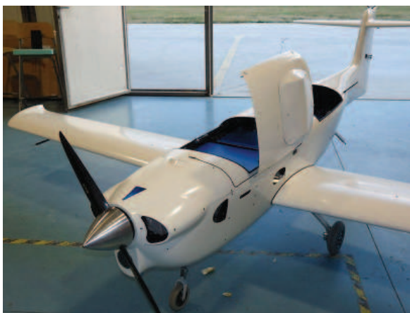
Fig. 11 K50 experimental UAV platform
