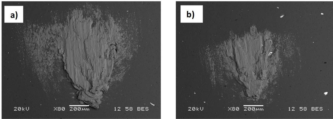
Figure 11 : Adhesive material on the pin after sliding on a) Reference-Ti6Al4V, b) EBM-Ti6Al4V
