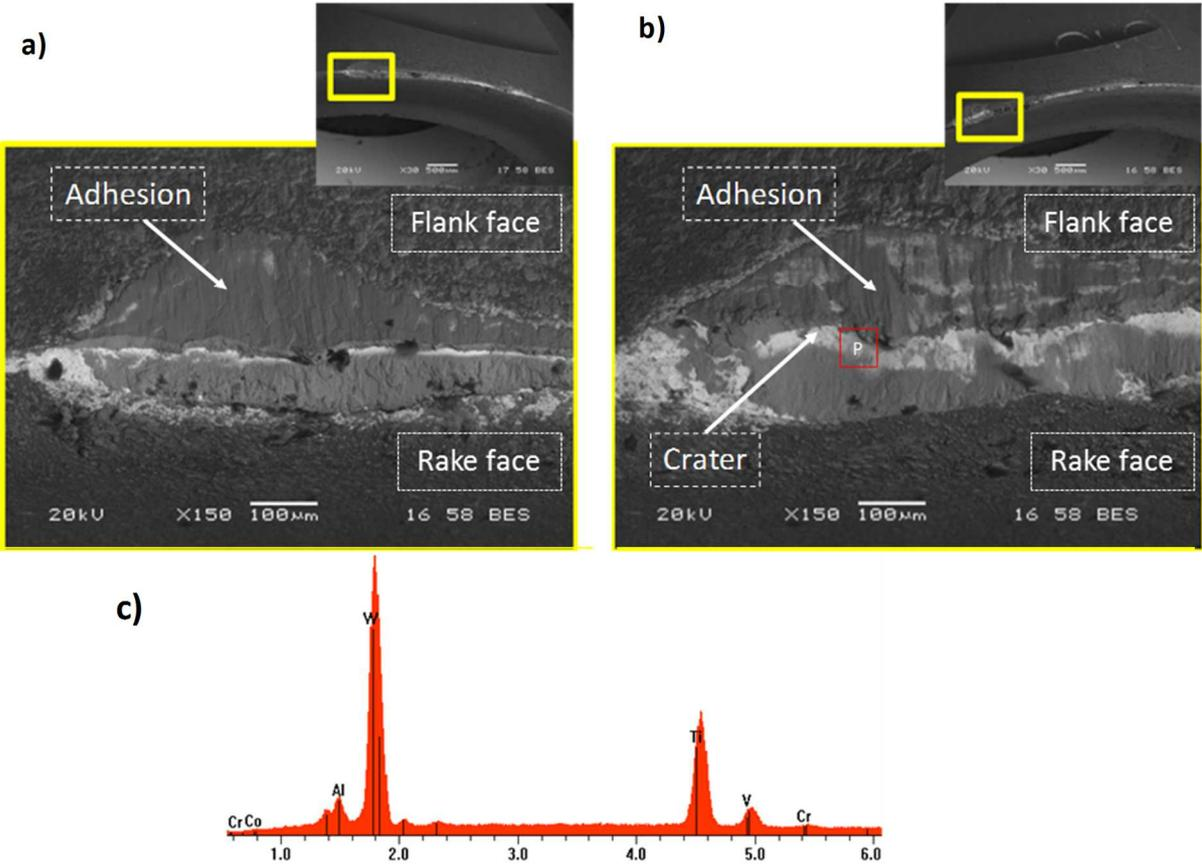
Figure 14 : Backscatter Images of Worn cutting edges at the end of tool life ( $V_b = 0.3 \text{ mm}$ ) after machining (a) Reference Ti6Al4V, (b) EBM – Ti6Al4V, (c) EDAX analysis at point P showing a high concentration of tungsten (W) of the substrate.
