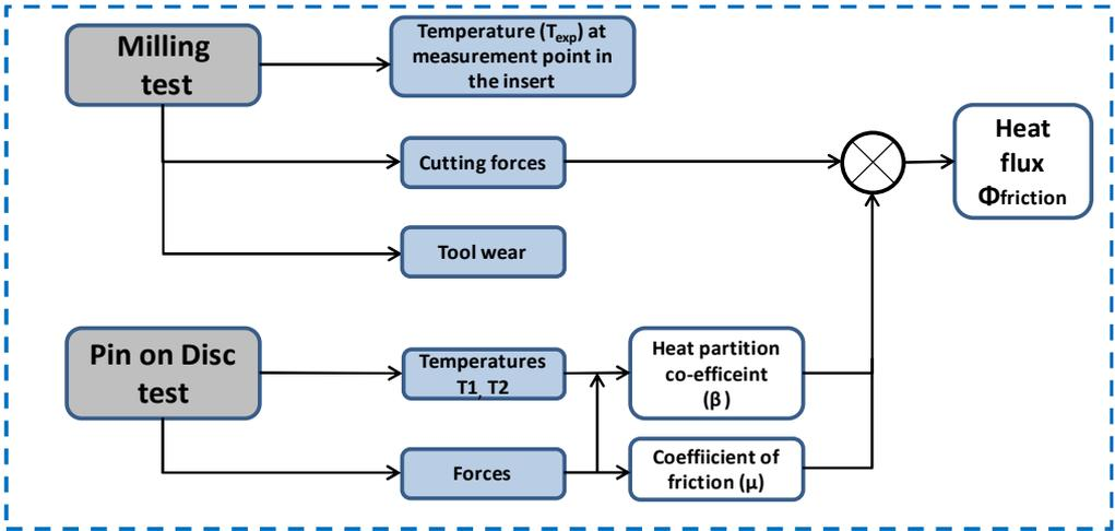
Figure 2 : Schematic representation of Hybrid method.
