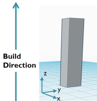
Figure 3 : Build direction of the EBM-Ti6Al4V samples.
