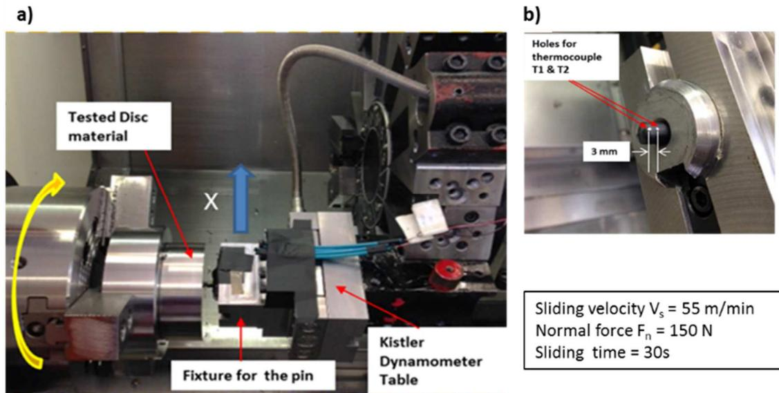
Figure 6 : Pin on Disc experimental set up.
