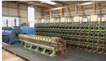
Fig. 2. Principle diagram of an electromagnetic launcher (railgun) and picture of the PEGASUS launcher (10 MJ).
