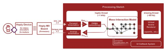
Figure 5: Full user-model interaction chain for non-audio haptic simulations. The kinematic calculations, physical computation and position/force I/O are all performed in a haptic thread, running at 1 kHz. The model is rendered at a lower rate in the draw() method.
