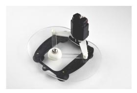
Figure 1: The 2-DoF Haply force-feedback device
