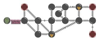
Figure 3: Representation of a mass-interaction model, composed of different types of mass and interaction elements.
