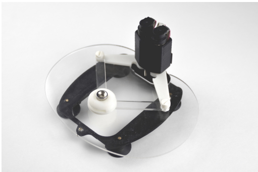
Figure 1: The 2-DoF Haply force-feedback device
