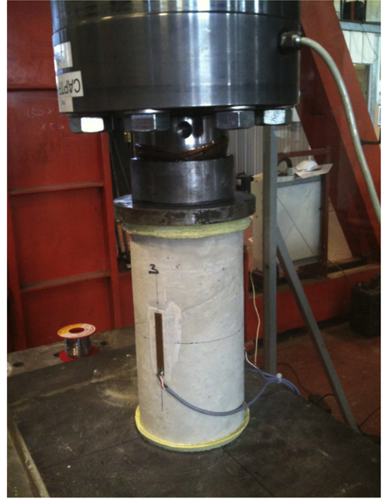
Fig. 3. Set up for cyclic test.
