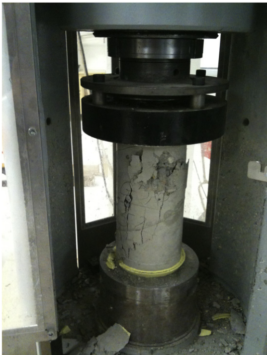
Fig. 5. A ramp test to measure compressive strength.
