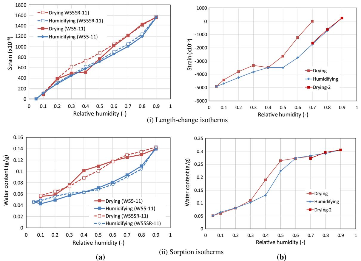
**Fig. 5** Length change isotherms (i) and sorption isotherms (ii) for samples W55-11, W55-SR-11 (a) and for the monolithic MCM-41 sample obtained by compaction (b). The data for samples W55-11 and W55SR-11 are from Ref. [13]
