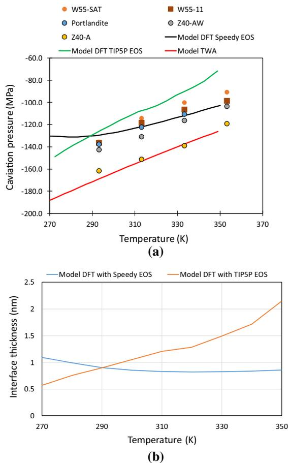
**Fig. 2** **a** Cavitation pressure measured on the various samples and predicted by modeling. Lines are cited from Herbert et al. [25]. Here, the experimental cavitation pressure is calculated by using the relative humidity at the beginning of sudden drop in desorption branch and Kelvin equation. **b** Liquid–vapor interface thickness calculated with DFT models. Data are cited from Caupin [23]
