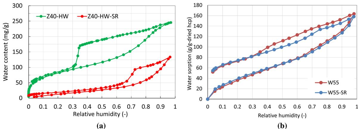
**Fig. 3** Modification of the adsorption isotherm by addition of a shrinkage reducing agent (SRA) in zeolite sample (a) and Hcp sample (b) (data is cited from Maruyama et al. [48]). The addition of SRA shifts the PSSD to larger relative humidities, i.e., up to about 0.7
