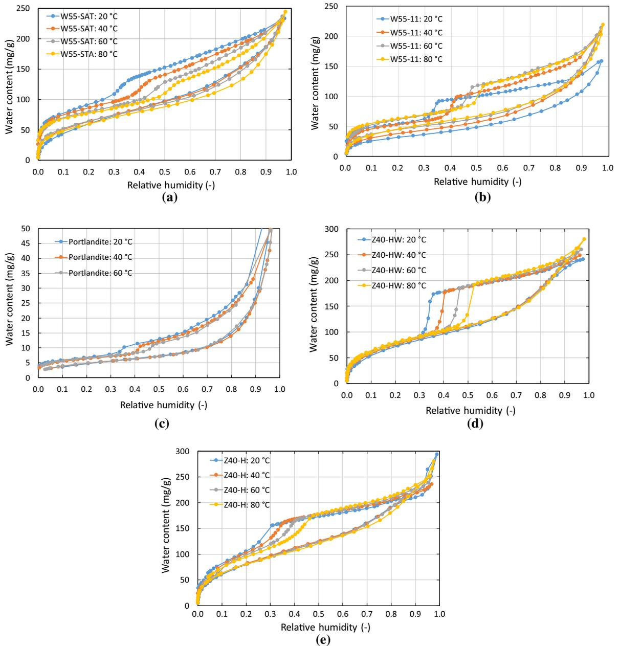
**Fig. 1** Sorption isotherms measured at various temperatures, showing that the relative humidity at which a sudden drop of adsorbed amount is observed on the desorption branch depends on temperature: **a** Saturated hardened cement paste (W55-SAT),
