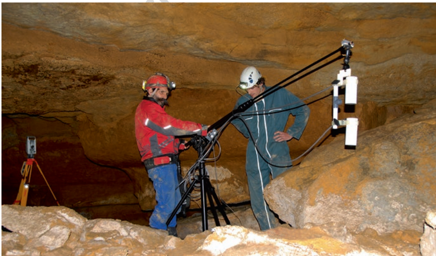
Fig. 9.11 View of the 3D magnetic prospecting device inside gallery no. 40. (Photograph: A. Burens)
