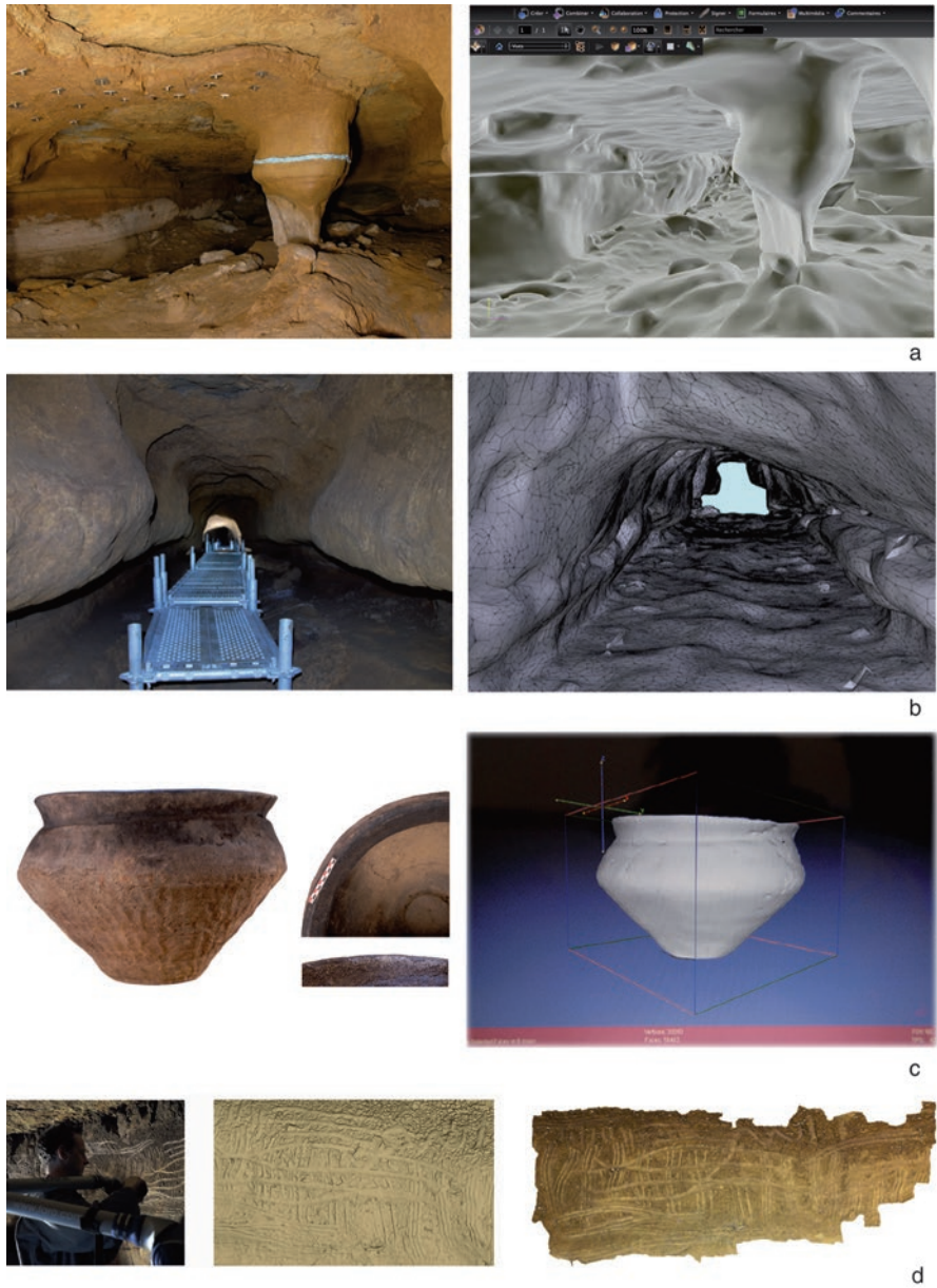
Fig. 9.5 3D recording of archaeological and geological information from the site based on terrestrial laser scanning, digital photogrammetry and spatial imaging system: (a) Image of gallery no. 13 of the cave (left) and its 3D model in PDF 3D format for visualisation in Adobe Reader (right), (b) Image of gallery no. 18 (left) and its 3D model in PDF 3D format (right), (c) 3D recording of a Bronze Age vessel from the cave, coated with the charred remains of animal fat, (d) 3D recording of the main decorated panel from gallery no. 13 (S. Guillemain, P. Grussenmeyer and A. Burens)
