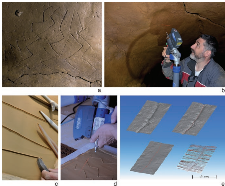
Fig. 9.8 3D recording of a decorated panel from gallery no. 10 and its experimental duplicate with the FARO ScanArm : (a) View of the decorated panel, (b) 3D recording of the decorated panel by TLS with the FARO ScanArm , (c) Preparation of experimental duplicates with different tools, (d) Scanning the experimental duplicate used as reference, (e) View of the section of the finest carvings from the decorated panel (A. Burens, S. Guillemin and P. Grussenmeyer)
