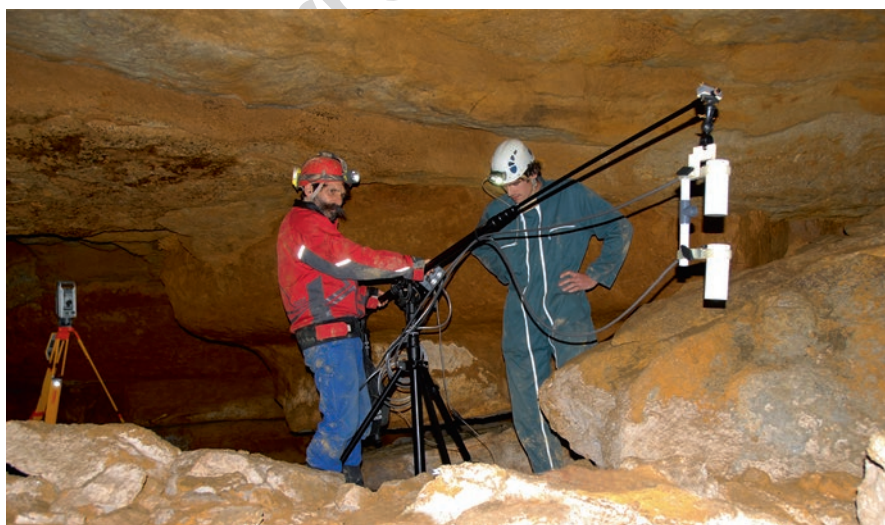
Fig. 9.11 View of the 3D magnetic prospecting device inside gallery no. 40. (Photograph: A. Burens)
