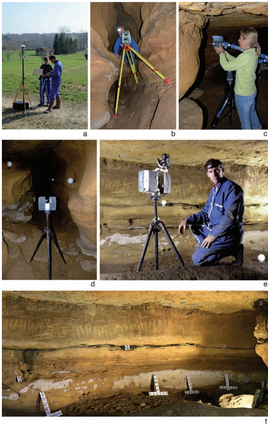
Fig. 9.4 Recording of the total network of galleries by surveying techniques and terrestrial laser scanning (TLS). The cave is linked to the above terrain thanks to surveying techniques (total station underground and GPS measurements in the field): (a) GPS measurements, (b) Surveying techniques by total station, (c, d) TLS, (e) TLS combined with photogrammetry, (f) Photogrammetry. (Photographs: A. Burens)
