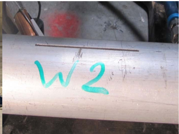
Figure 2: detailed view of the machined slot
