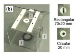
Figure 2: (a) Description of the submerged release apparatus and (b) Illustration of the transparent box to experiment gravity release in the water column
