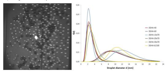
Figure 4: (a) Picture of DEHA droplet at the top of the column and handmade analysis of droplet diameter. (b) Droplet size distribution in the water column.
