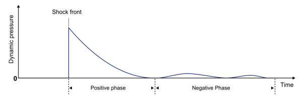
Figure 1: Dynamic pressure profile behind a shockwave at a constant location
