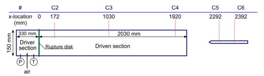
Figure 2: Shock tube configuration with sensors
