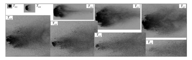
Fiugure. 5: Fragmentation of a 0.8 mm diameter droplet at different dimensionless time.
