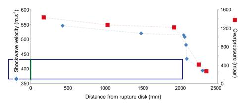
Figure 3: Shock tube velocity and overpressure over distance from rupture disk
