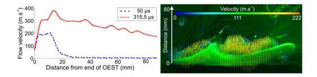
Figure 4: Flow velocity at different time after exit from OEST (left) – PIV analysis extraction at 50 µs (right).
