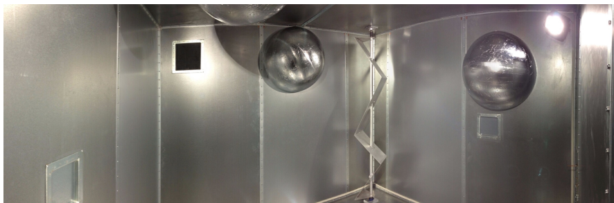
Fig. 1 180-degree photograph of the chaotic RC at ESYCOM. The commercial RC consists in a rectangular metallic cavity of dimensions W = 2.95 m, L = 2.75 m and H = 2.35 m and was modified by placing 3 hemispheres with radii of 40 cm (one at the ceiling and two on adjacent walls). The mechanical stirrer in the far corner can be seen.
