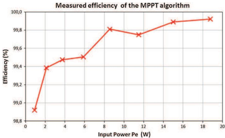
Fig. 13. Measured power efficiency of the P&O algorithm.
