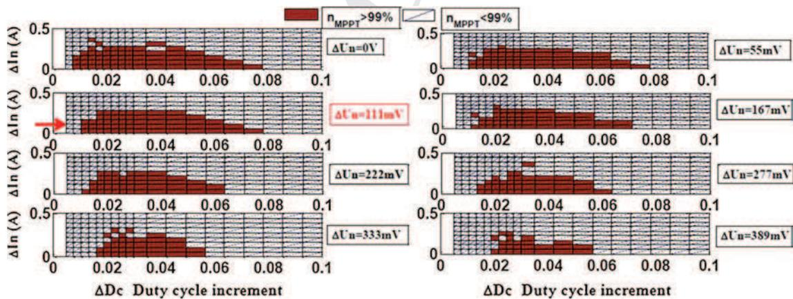
Fig. 9. Influence of noise ( $\Delta I_n$  and  $\Delta V_n$ ) on the energy efficiency of the P&O algorithm.
