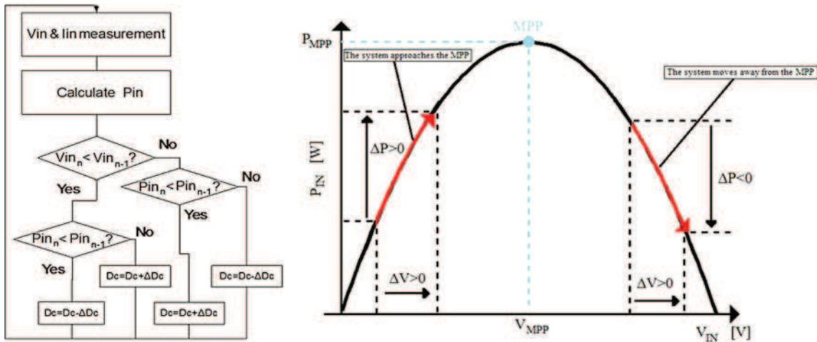
Fig. 7. Principle of MPPT with its algorithm.
