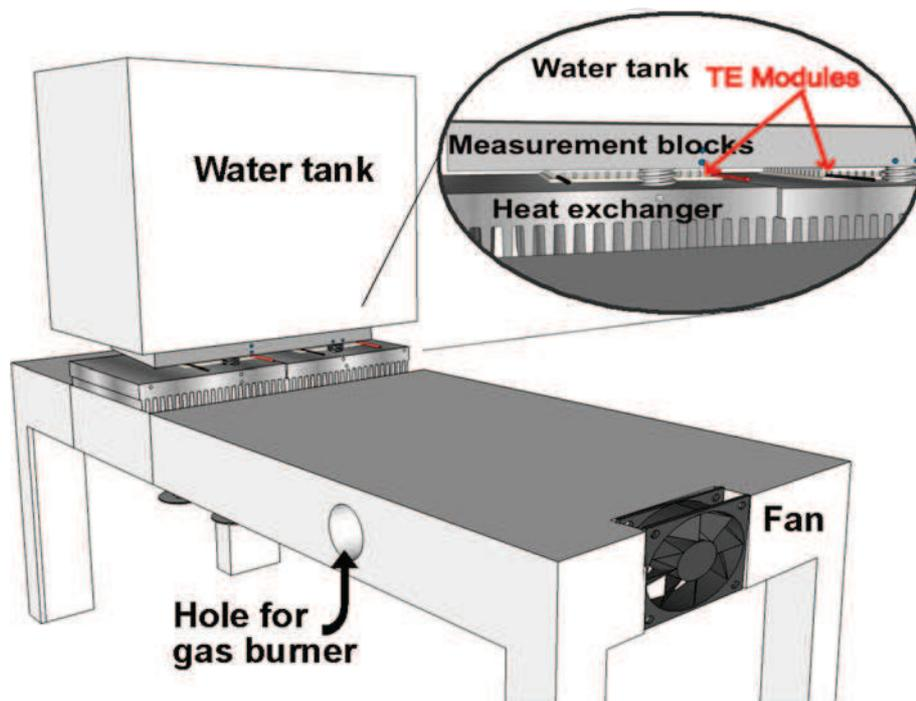
Fig. 14. Test bench for simulating the stove.
