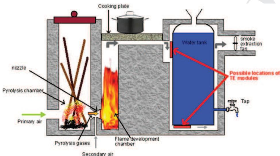
Fig. 2. Planète Bois cooking/water heating stove design.
