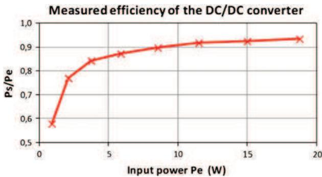
Fig. 11. Electronic power efficiency of the DC/DC converter.
