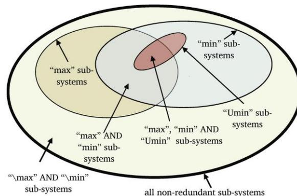
Fig. 42 How the filters “\max”, “\min” and “\umin” work.<sup>201</sup>
