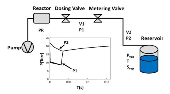
Fig. 5: Schematic of vapor dosing system for a liquid precursor used in the systems by Encapsulix (PR: reactor pressure,  $P_{vap}$ : Precursor vapor pressure, T: temperature,  $S_{vap}$ : Precursor surface area. The graph shows the simulated pressure (P1 and P2) in the two volumes (V1 and V2) during and immediately after a pulse.
