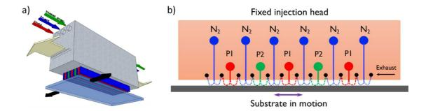
**Fig. 3.** a) Scheme of a SALD close-proximity head in which the substrate is oscillated below the slots through which the different precursors are continuously injected. B) Side view of the head-substrate gap showing the paths of the different flows that take place for the small gap used, which ensure no precursor crosstalk.
