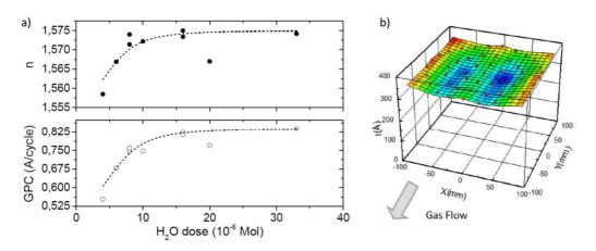
**Fig. 18**. 25 nm thick  $Al_2O_3$  film made in a PPWR Infinity 200 reactor, 3 s/cycle, 90°C.Left: a) optical index (n) and GPC vs. the  $H_2O$  dose; b) non-uniformity of the alumina layer measured on a 200 mm Si wafer
