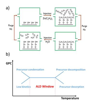
**Fig. 1.** a) Scheme of the Atomic Layer Deposition (ALD) process for the deposition of ZnO, showing the alternative steps: a first precursor (DEZ, diethylzinc) is injected and a purge occurs followed by the injection of the second precursor (water) and so on. b) Scheme of the typical Growth per Cycle (GPC) as a function of temperature in ALD.
