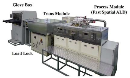
Fig. 15. Photograph of the fast spatial ALD system used by Choi et al. to encapsulate OLED panels.[71]
