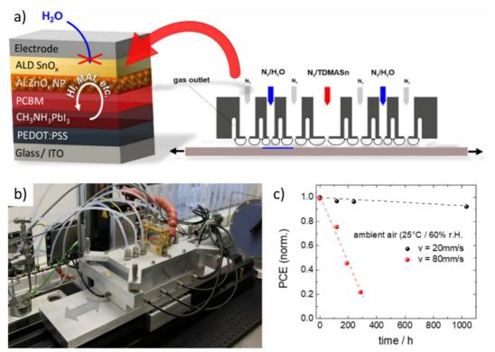
**Fig. 17.** a) Schematic of the SALD assembly used to deposit a  $SnO_x$  layer as part of a perovskite solar cell stack; [79] b) Plasma SALD system inside a globe box for the deposition of  $SnO_x$  layers for solar cells based on hybrid perovskies; c) Normalized photoconversion efficiency (PCE) vs. time of storage in ambient air (25 °C, 60% RH) for solar cells with SALD  $SnO_x$  layers grown at 20 and 80 mm/s, respectively. (Images courtesy of Prof. T. Riedl);
