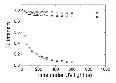
**Fig.14.** Evolution of the normalized fluorescence (FL) intensity, under constant UV light, in laboratory atmosphere, of (squares) an  $Al_2Q_3$  thin film and an  $Al_2Q_3$  thin film encapsulated with 25 nm  $Al_2O_3$  deposited by low temperature ALD (90 °C) in (triangles) a Savanah 200 standard cross-flow reactor (30 s/cycle) and (circles) in an fast-ALD Infinity 200 PPWR system from Encapsulix (3 s/cycle); thickness of  $Al_2Q_3$  films is 100 nm.
