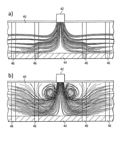
**Fig. 4.** Computational Fluid Dynamics (CFD) study of the development of a vortex in a gas injection volume at different flow speeds.a) low flow rate, aproximately 133 sccm. b) High flow rate, aproximately 1333 sccm. [82]
