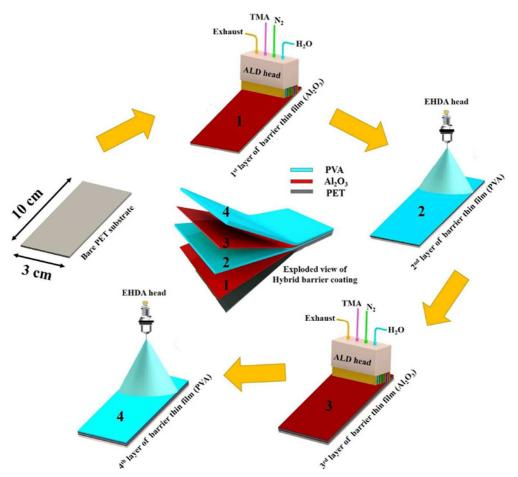
Fig. 22. Flow process diagram of hybrid multilayer barrier coating containing bare PET substrate. [70]
