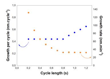
Fig. 12. Evolution of the SiO<sub>2</sub> growth per cycle and growth rate depending on cycle length in FAST deposition mode.
