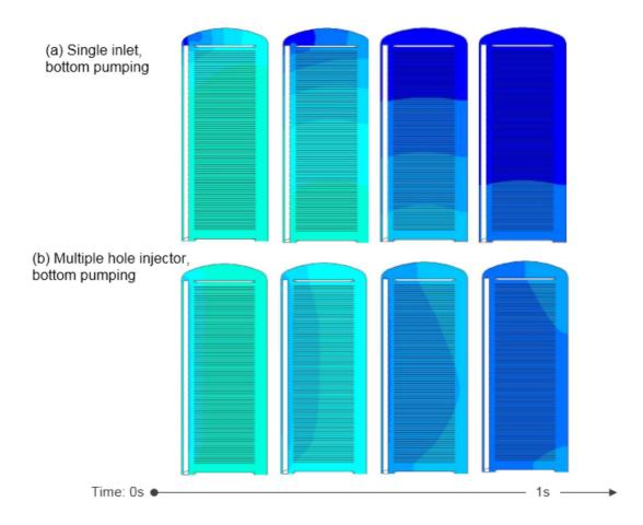
**Fig. 2.** Contour plots of precursor (TiCl<sub>4</sub>) partial pressure at different times after precursor injection in two similar batch reactors. a) Single inlet reactor. b) Multiple inlet reactor. Reprinted from ref. [24] with permission.
