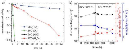
**Fig. 20.** a) Normalized conductivity upon aging under damp heat conditions (85 °C and 85% RH) of 200 nm thick ZnO, AZO, and SnO<sub>x</sub> films (grown at 150 °C) using  $O_3$  or  $H_2O$  as oxidants; b) electrical conductivity, carrier density and electron mobility of SnO2 deposited by HT PE-ALD
