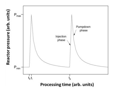
Fig. 8. Evolution of the pressure in the reactor during a pulsed pressure CVD deposition.
