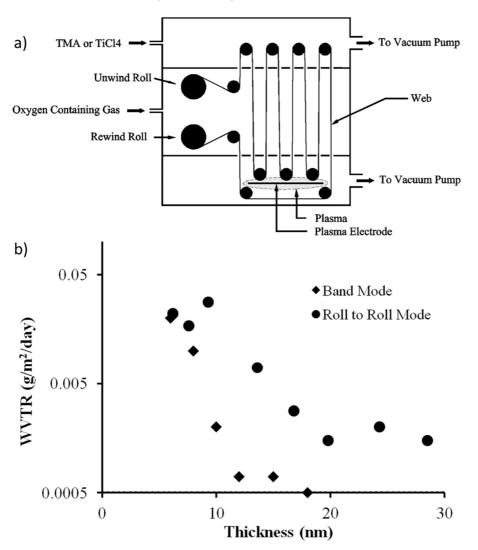
**Fig. 21.** a) Schematic Representation of the LOTUS Applied technology roll-to-roll (R2R) reactor configured for plasma-based SALD; b) Chart of water vapor barrier performance for ALD TiO<sub>2</sub> films on "generic" industrial grade PET, deposited by substrate translation.
