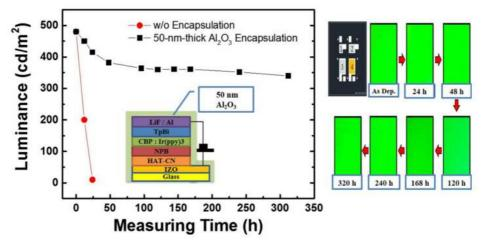
Fig.16. Emission lifetime evaluation of Al<sub>2</sub>O<sub>3</sub> encapsulation on an OLED panel.
