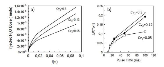
**Fig. 6.** a) Simulated of precursor doses injected vs. time after valve opening, for different dosing valve opening times; b) Experimental injected doses expressed as variation in pressure vs. time after valve opening, for different dosing valve opening times.
