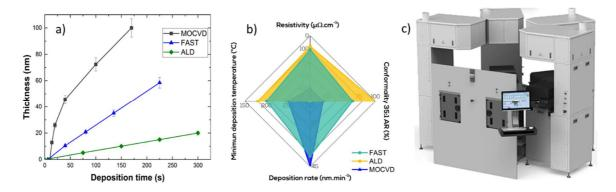
**Fig. 10.** a) Variation of TiN deposition rate from TDEAT and NH<sub>3</sub> by ALD, MOCVD, and FAST techniques. b) Comparison of ALD, CVD and FAST deposition techniques for the deposition of TiN using the same precursors and temperature. c) FAST reactor cluster from KOBUS used to perform the deposition of TiN in the three different modes.
