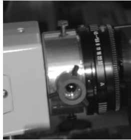
Fig.3: The interferometric head, showing lens holder
