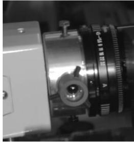
Fig.3: The interferometric head, showing lens holder
