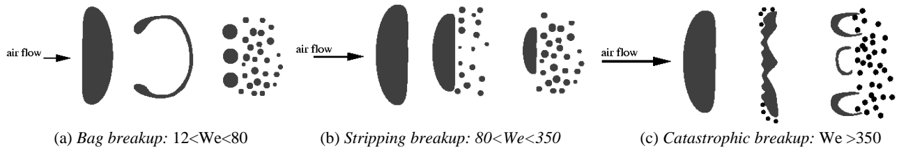
Figure 2: Schematic representation of droplet breakup mechanisms [7]
