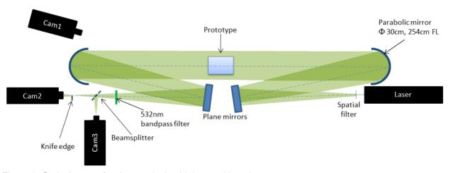
Figure 3: Optical set-up for dust explosion high speed imaging
