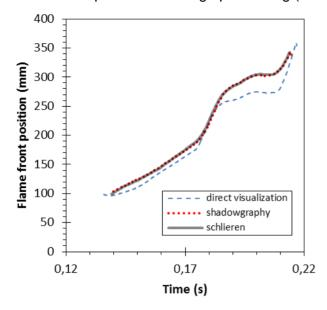
Figure 5: Evolution of the flame front position for the upper zone of visualization
