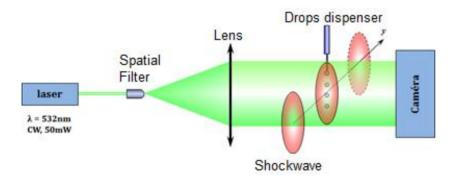
Figure 6: Set-up for in-line digital holography on falling droplets with shockwave.
