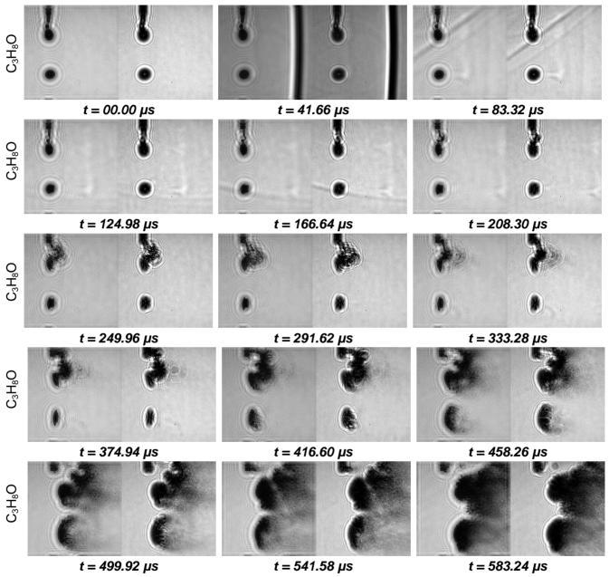
Figure 7: TRILDHI Time code images for ethanol: unitary magnification 20µm/pixel, 512x512pixels, 24890fps
