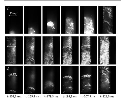
Figure 4: Flame propagation velocity on the upper part of the prototype: by direct visualization (a), shadowgraphy (b) and schlieren (c). Time between images: 14ms
