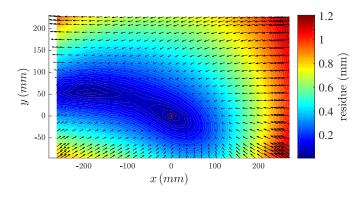
Figure 9: Residue between measurements and model without defect (nominal model)
