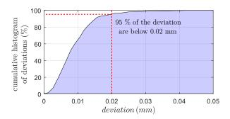
Figure 11: Cumulative histogram of deviations from Fig. 10 (in %).
