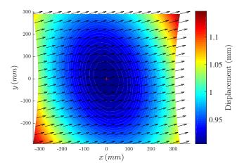
Figure 5: Influence on the nominal model of a unitary orientation defect of the laser source around  $\frac{1}{c_s^2}$  ( $\delta c_s = 1$  mrad).
