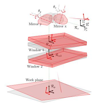
Figure 4: Optical chain parameterization with 30 assembly defects.
