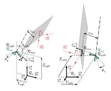
Figure 3: Mirrors parameterization details of the Fig. 2
