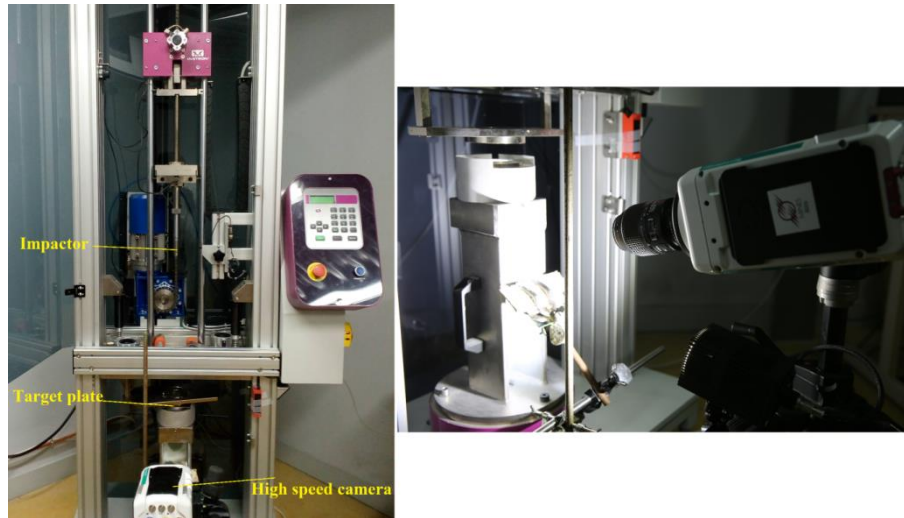
Figure 1 Drop tower setup for impact testing of composite plates
