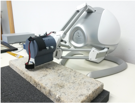
Figure 2: The data recording system. An accelerometer on a tool tip that is mounted on the force feedback device scans surfaces horizontally with a constant velocity of 80 mm/s.
